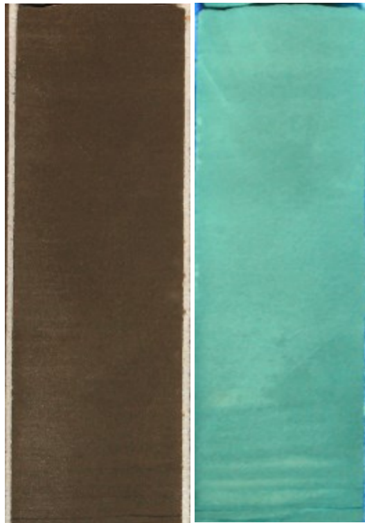
Figure 4.11: Core photography of Cleveland "C" Sandstone. Mid-Con Energy, J.A Jones #58 (1643-1644 ft.) (T.21N, R.8E, Sec.20, Pawnee Co., Oklahoma). Left: Plain light. Right: Ultraviolet light. Very fine- to fine-grained sandstone. Sedimentary structures (massive to planar bedding) are largely obscured by oil staining.
