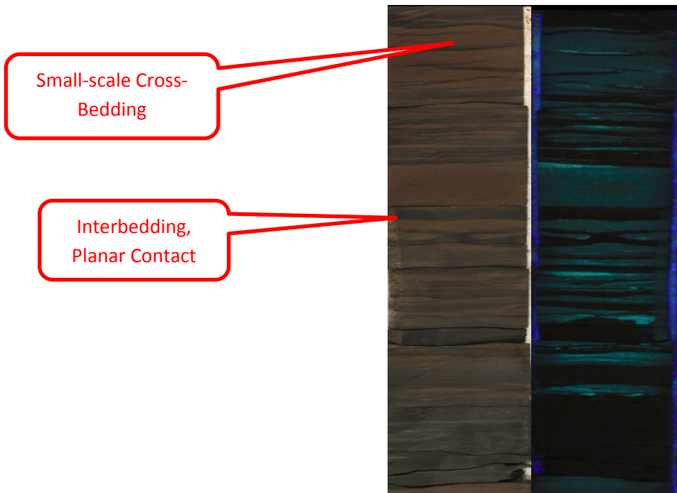
Figure 4.2: Core photographs of Cleveland “A” Sandstone. Mid-Con Energy, J.A Jones #58 (1581-1583 ft.) (T.21N, R.8E, Sec.20, Pawnee Co., Oklahoma). Left: Plain light. Right: Ultraviolet light. Interbedded to interlaminated, very fine-grained sandstone, and siltstone. Contacts mostly are planar (horizontal), but some beds-laminae show small-scale cross-bedding (ripple bedding).
