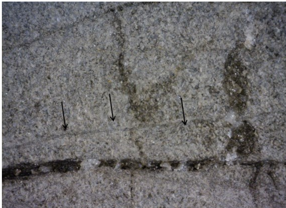
Figure 5.8: Enlargement of part of Figure 5.7. Black arrows point to a partly sealed fracture. Aperture of the fracture is approximately 1 mm. It is propped open by euhedral calcite crystals.
