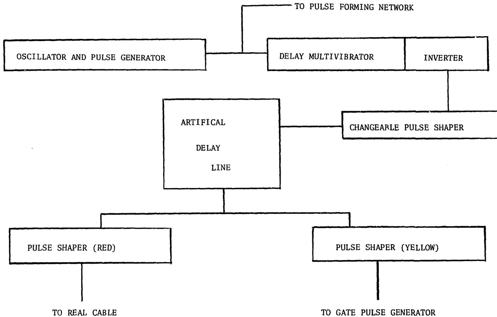
Figure 38. Block Diagram of Timer as Used with Combination System V and Preionization.
