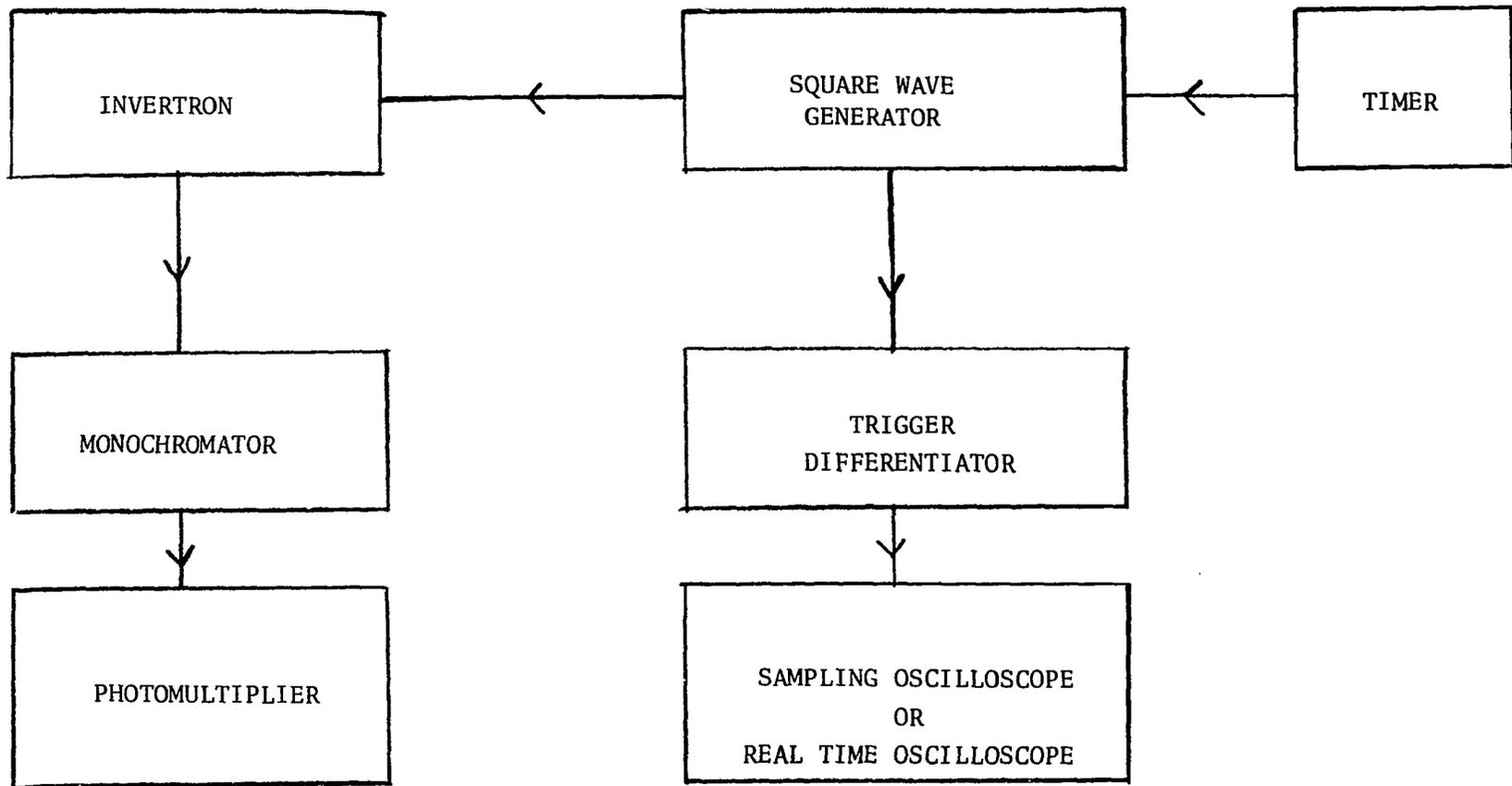
Figure 4. Combination System I or III: Direct View or Sampling Scope and Coaxial Cable.
