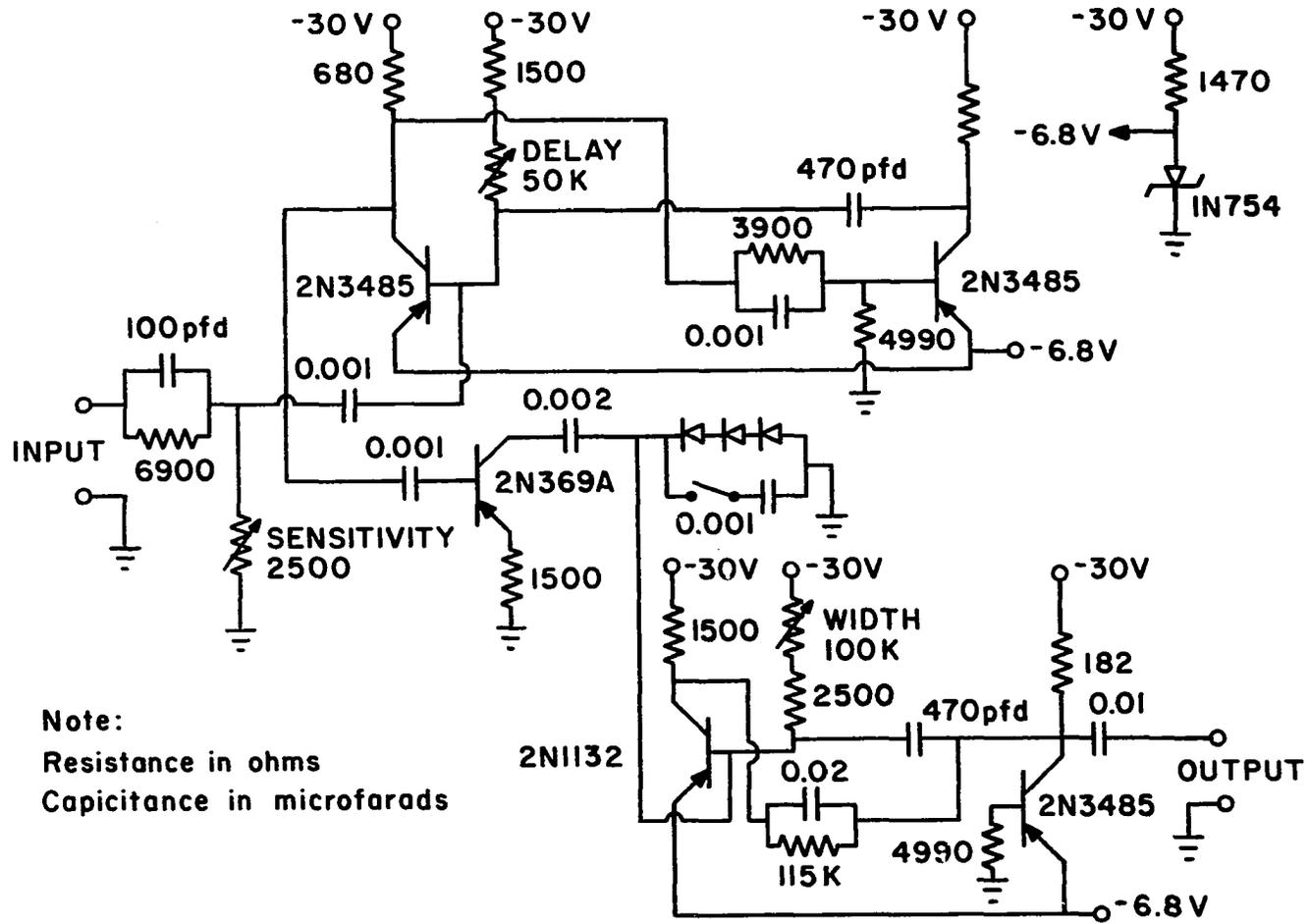
Figure 33. Gate Pulse Generator.
