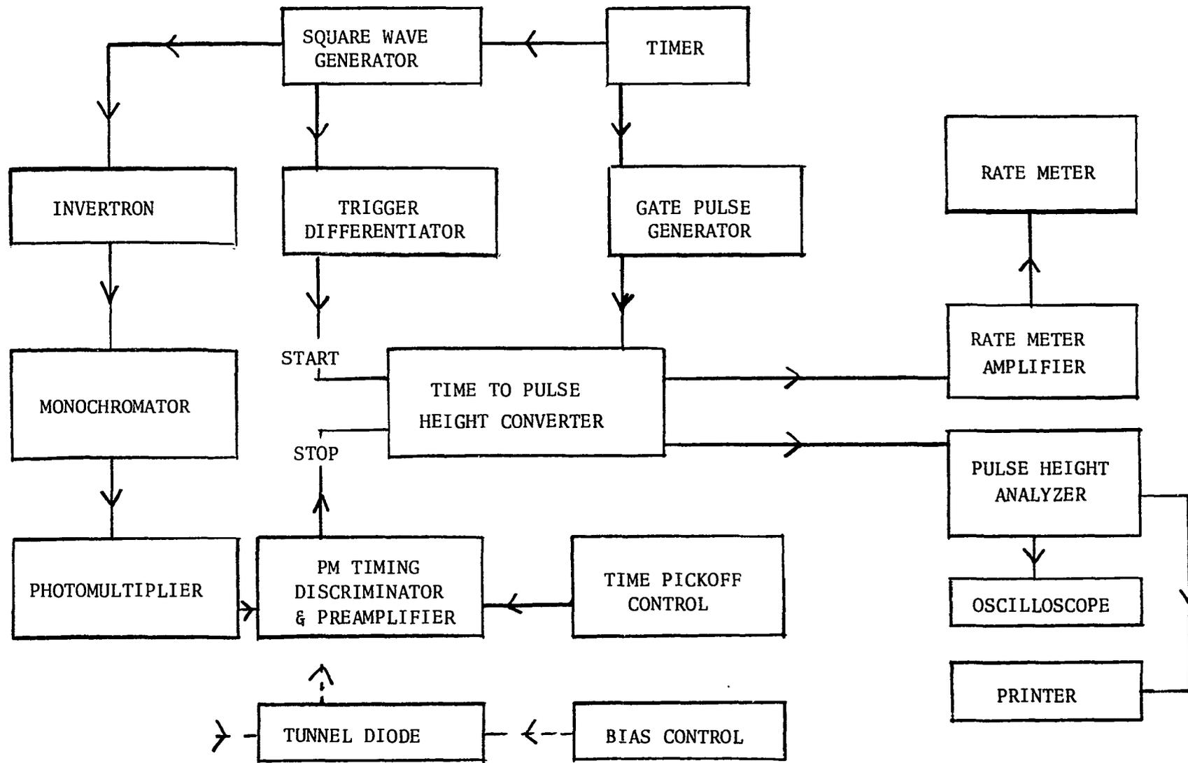
Figure 6. Combination System V: Delayed Coincidence and Coaxial Cable.
