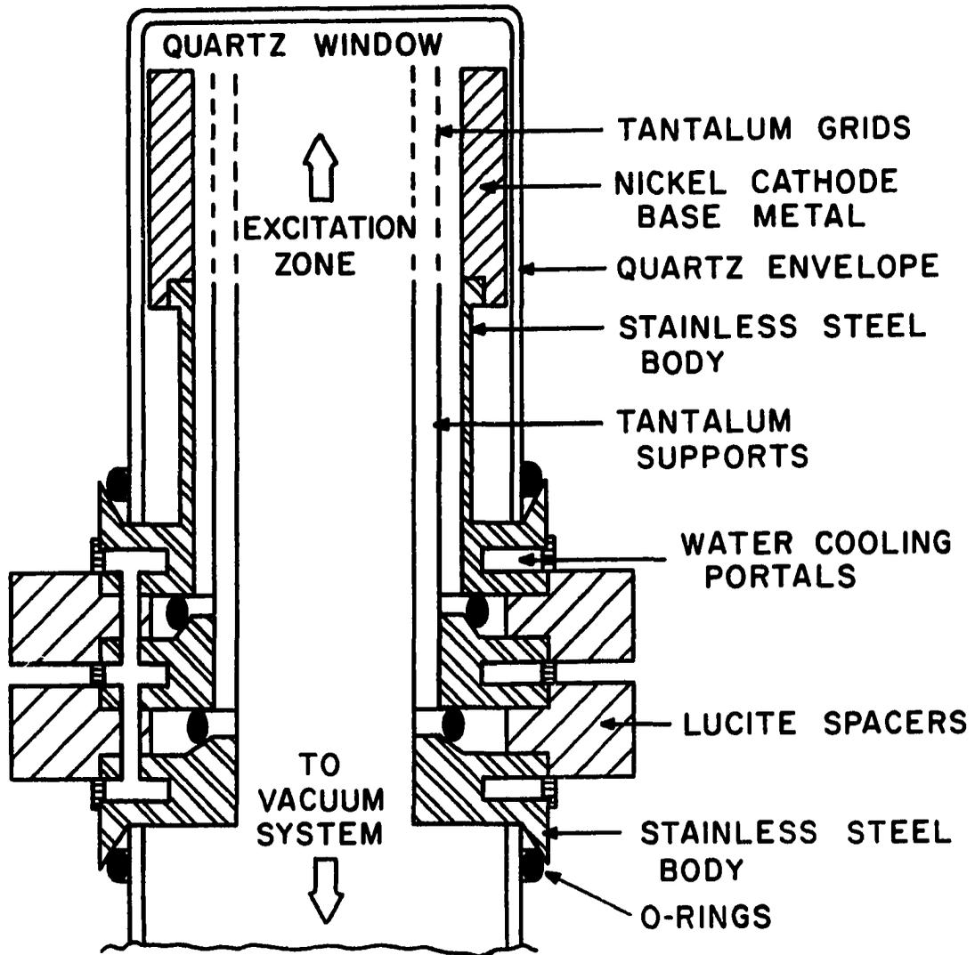
Figure 3. Cross Section of Invertron.
