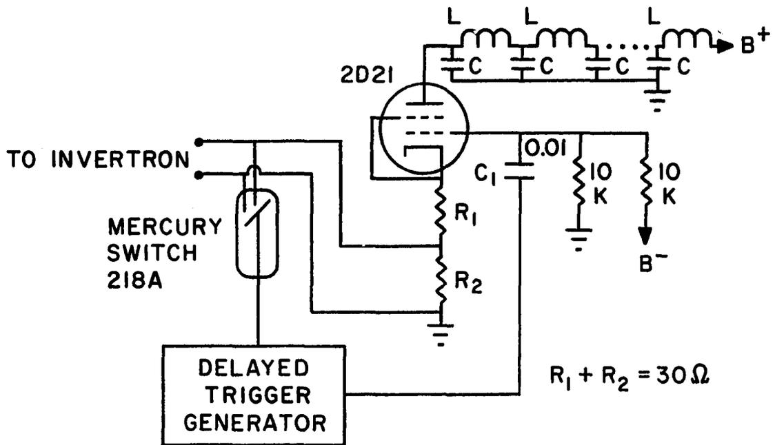
Figure 32. Mercury Switch and Pulse Forming Network.
