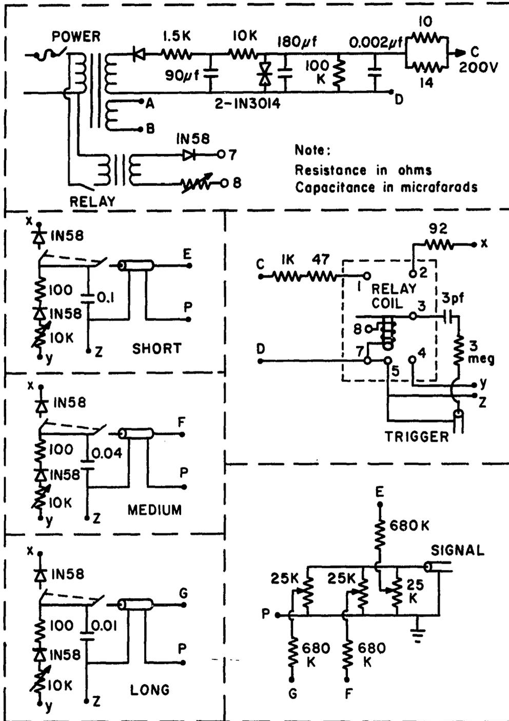
Figure 39. Exponential Function Synthesizer.
