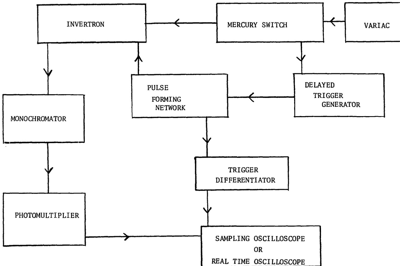
Figure 5. Combination System II or IV: Direct View or Sampling Scope with Mercury Switch.
