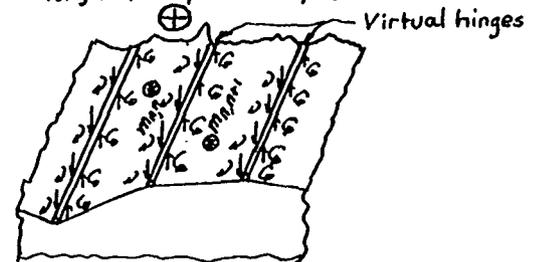
(c.2) Structure with virtual hinges for correction analysis.
