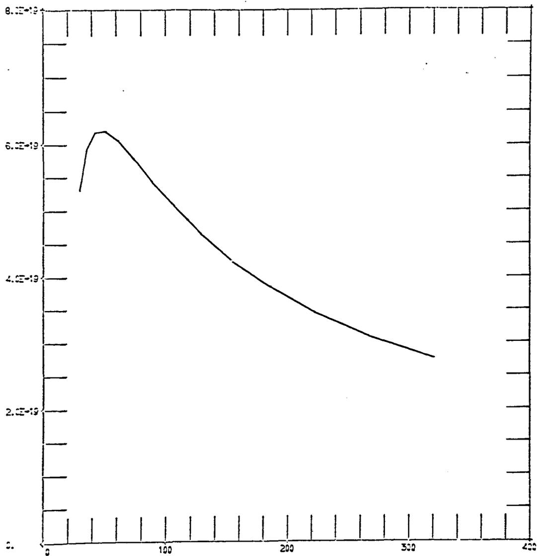
Figure A2. Cross section (cm<sup>2</sup>) vs Electron Energy (e)
