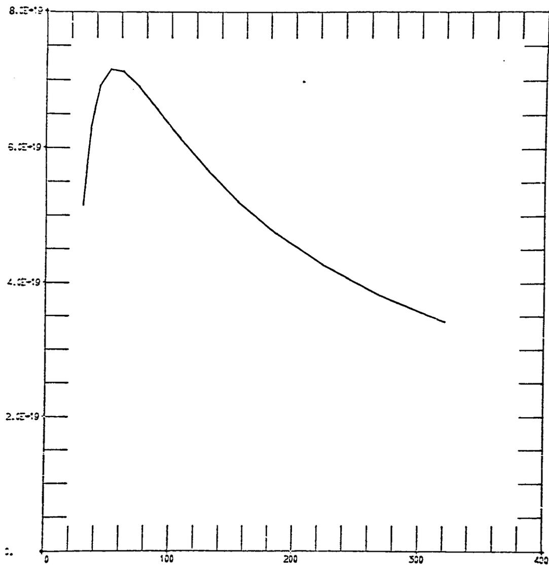
Figure A29. Cross section (cm<sup>2</sup>) vs Electron Energy (eV)
