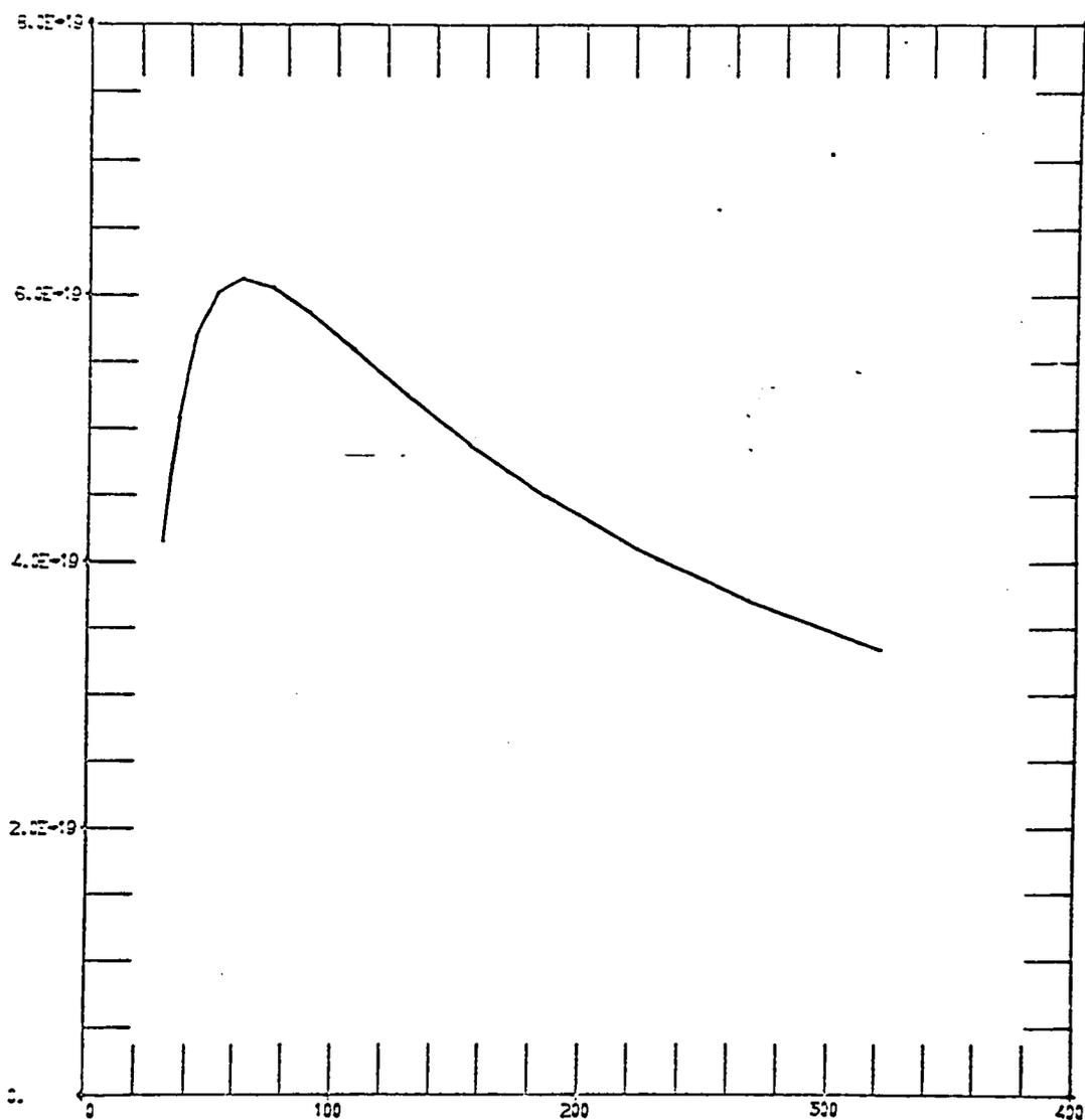
Figure A24. Cross section (cm<sup>2</sup>) vs Electron Energy (eV)
