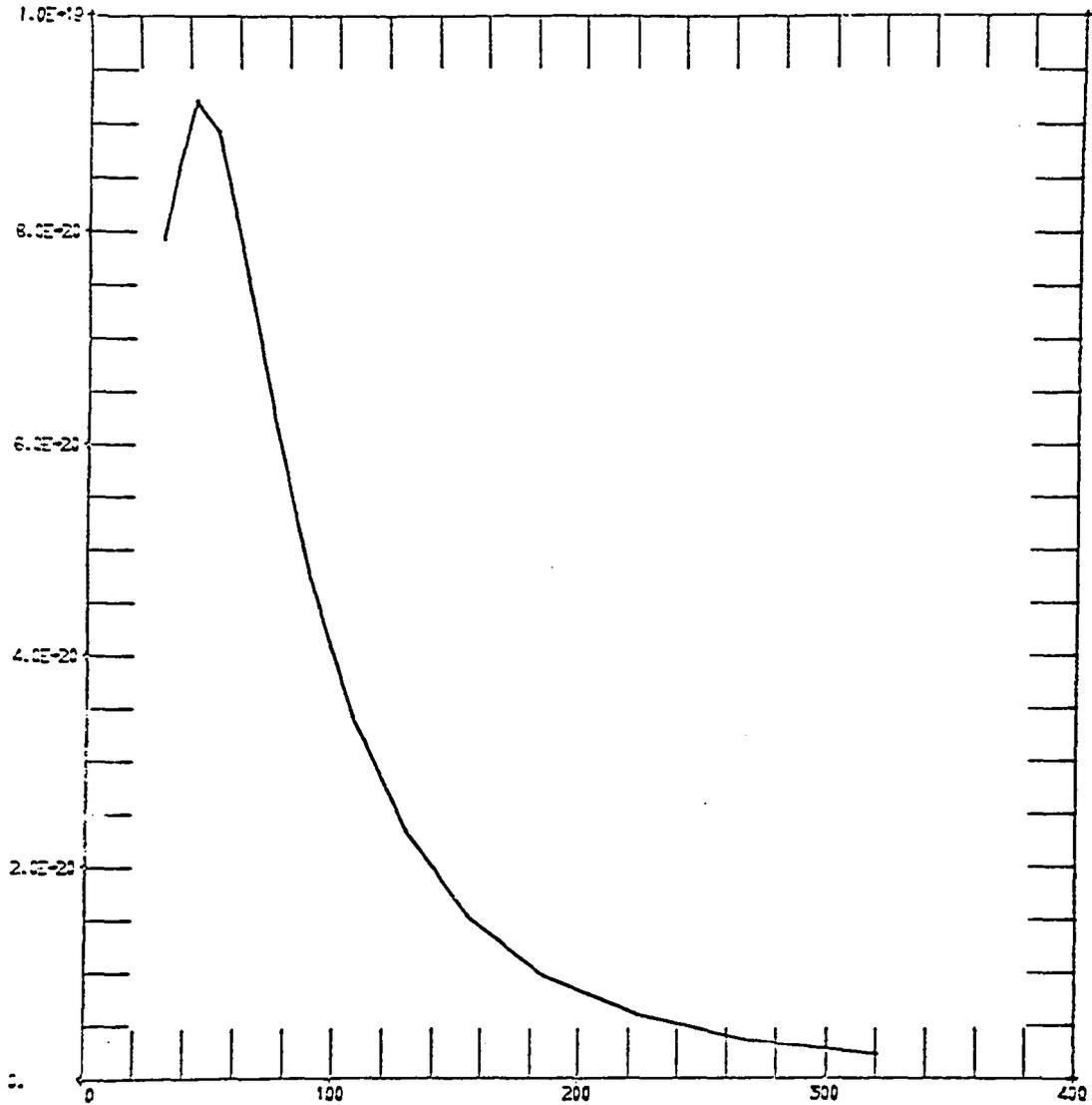
Figure A5. Cross section (cm<sup>2</sup>) vs Electron Energy (eV)
