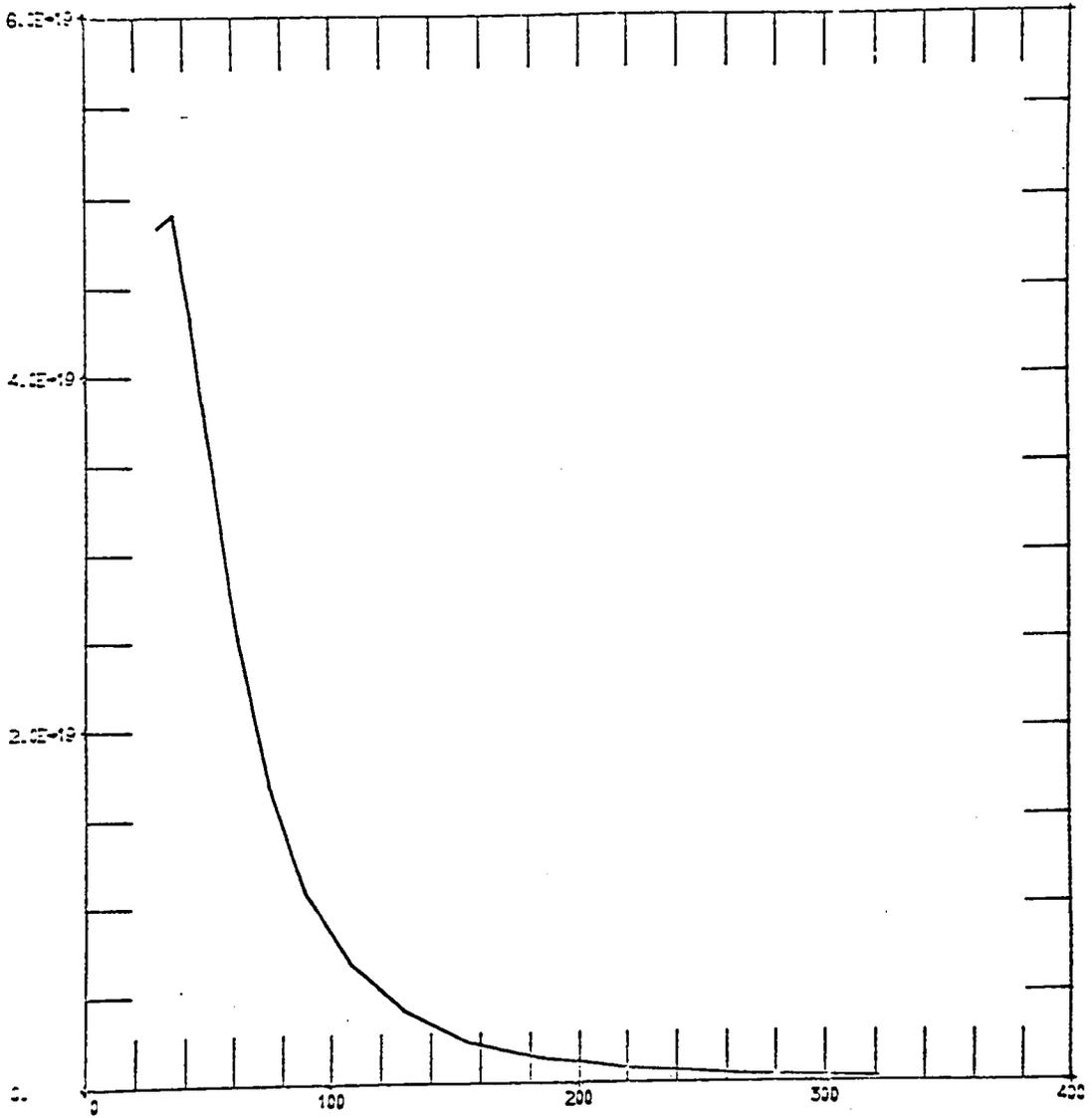
Figure A1. Cross section ( $\text{cm}^2$ ) vs Electron Energy (eV)
