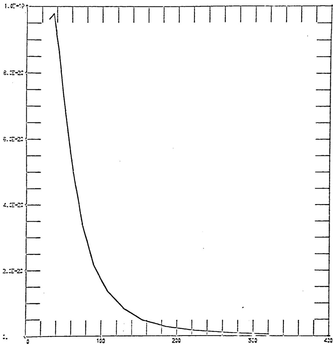
Figure A4. Cross section (cm<sup>2</sup>) vs Electron Energy (eV)
