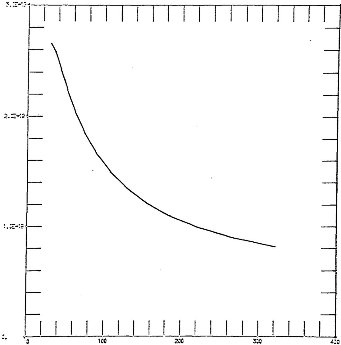
Figure A13. Cross section (cm<sup>2</sup>) vs Electron Energy (eV)
