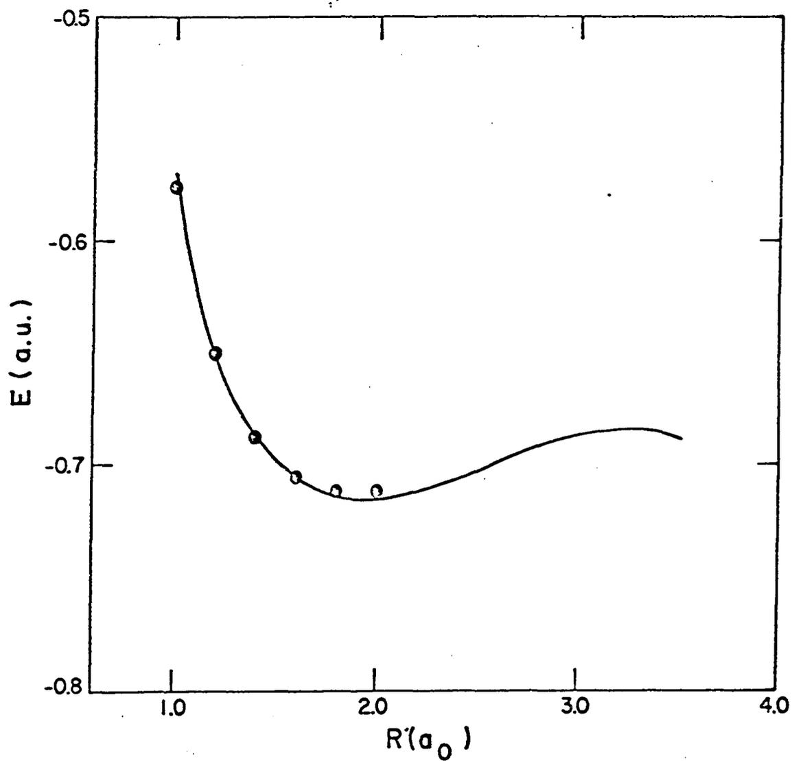
Figure 2. Electronic energies for the E state. The solid curve is the potential obtained by Davidson. The points represent the present results.
