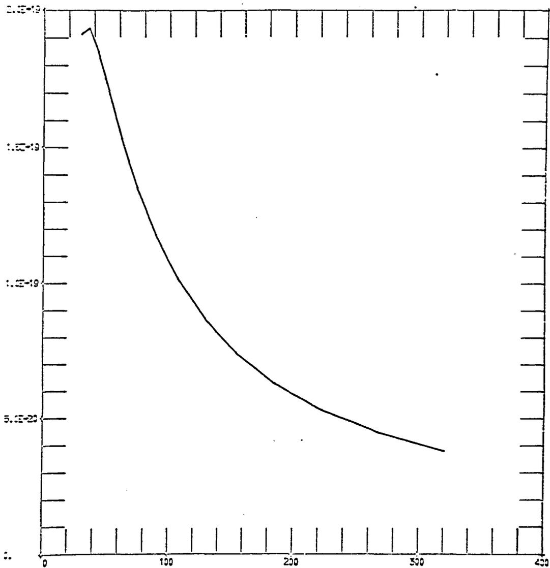
Figure A8. Cross section (cm<sup>2</sup>) vs Electron Energy (eV)
