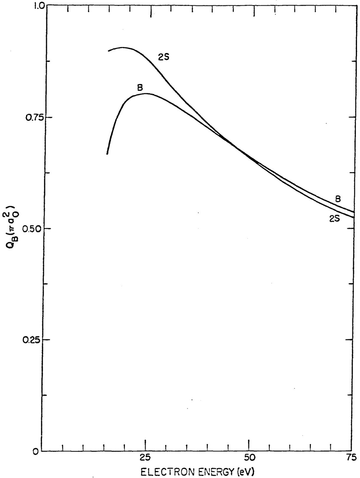
Figure 10. Total cross sections for the B state, as given by the two state close coupling and Born approximations.
