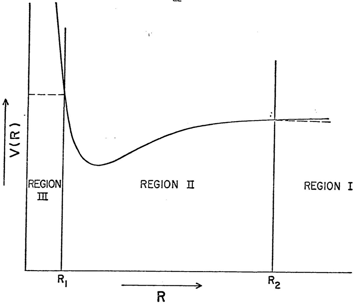
Figure 3. A typical potential curve. The solid curve illustrates the usual shape of  $V(R)$ .  $U(R)$  is given by the dashed lines, where it differs from  $V(R)$ .
