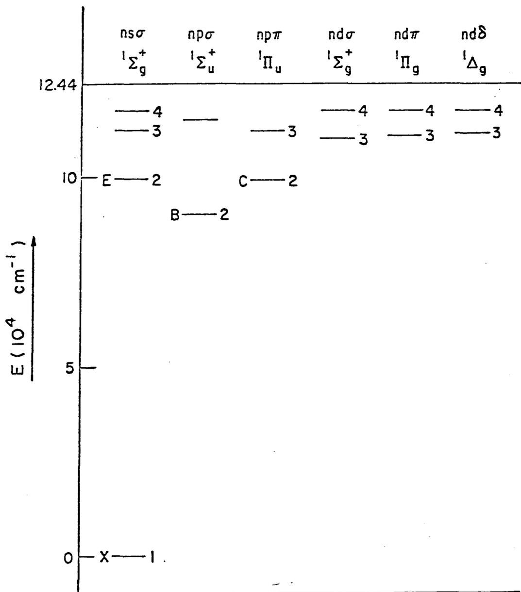
Figure 7. Electronic energy level diagram, showing the approximate position of the  $v = 0$  vibrational level of some of the singlet electronic states.
