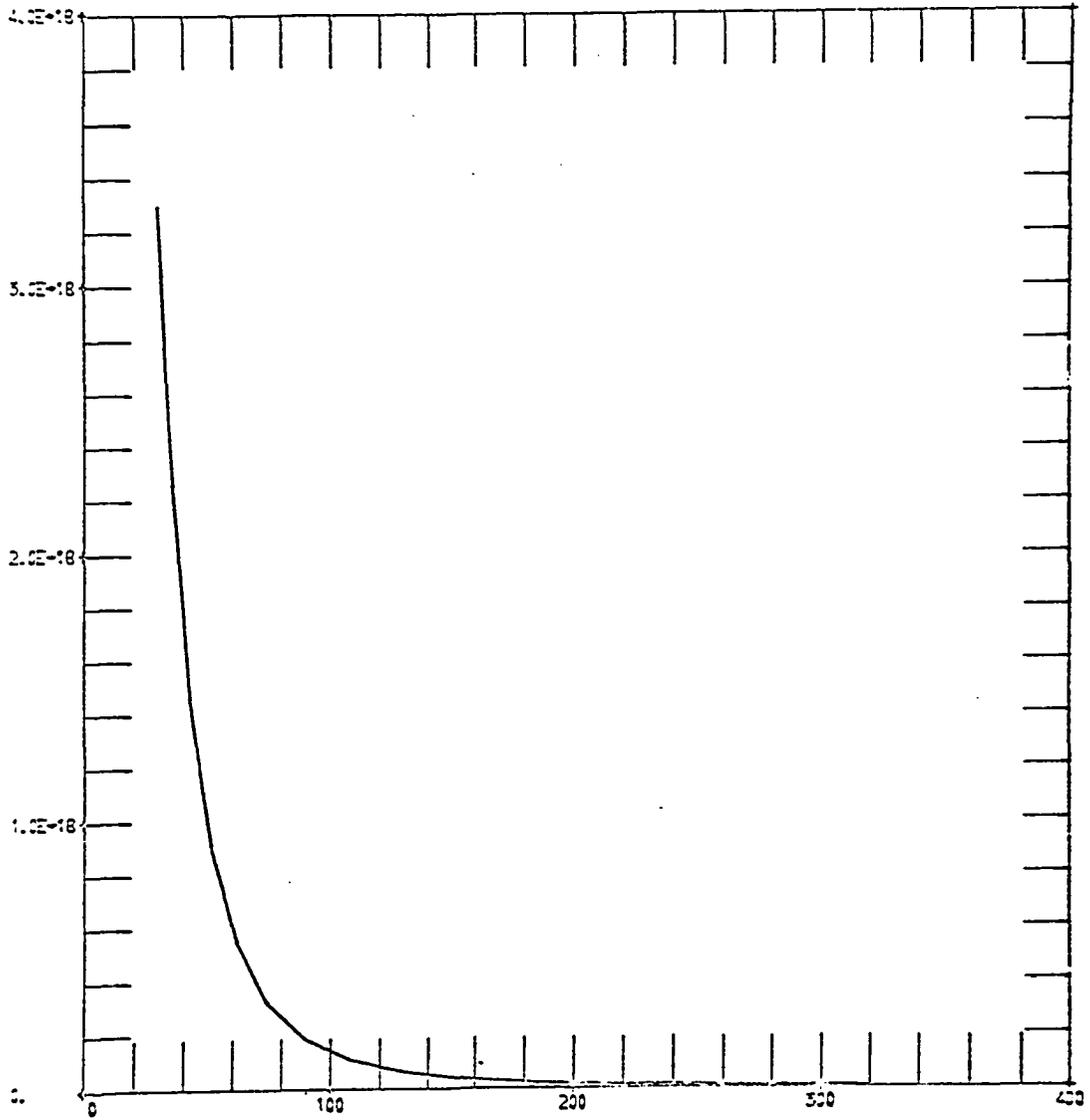
Figure A9. Cross section (cm<sup>2</sup>) vs Electron Energy (eV)
