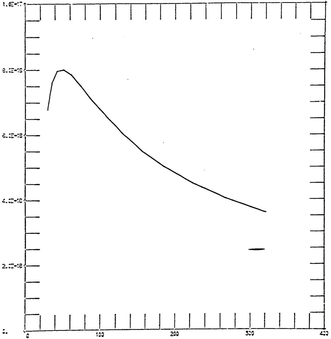
Figure A3. Cross section (cm<sup>2</sup>) vs Electron Energy (eV)
