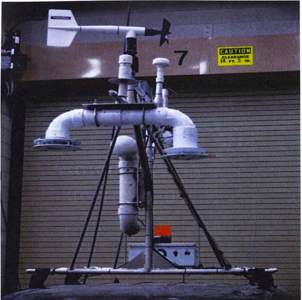
Figure 2: Mobile Mesonet showing mounting location and orientation of the U-tube. The picture was taken from the nose of the vehicle. The intake is on the passengers (left) side of the vehicle while the exhaust is on the drivers (right) side. The mounting location puts the U-tube above the front windshield to maximize airflow without distortions from the rack, but is high enough to be removed from reradiation of energy off the vehicle roof.
