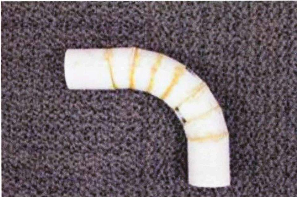
Figure 8: Inner tube created by piecing several sections of 1 inch (25.4 mm) diameter tube. Each section was created from a straight pipe cut at opposing 7.5° angles.
