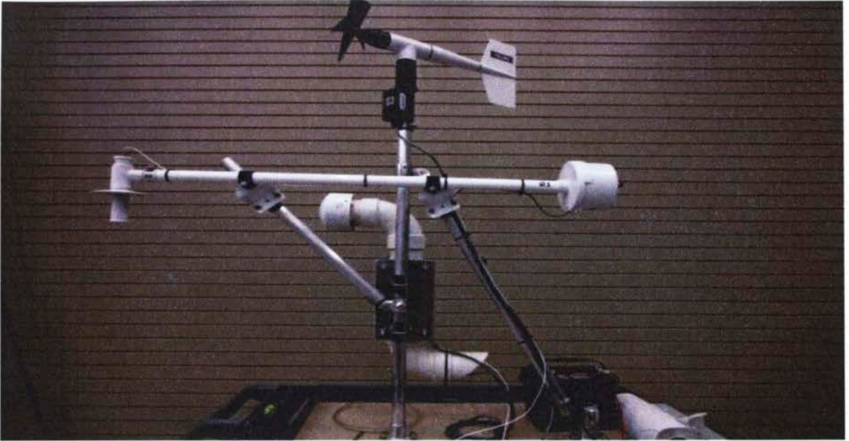
Figure 1: Cart mounted rack created for time constant study. Rack pictured shows mounting of RM Young Wind Monitor, J-tube, and RM Young 43408. The orientations of the instruments are the same as is used on the Mobile Mesonet. The cart used for the U-tube portion of this test was identical to the cart pictured above, except with the U-tube mounted to the side of the J-
