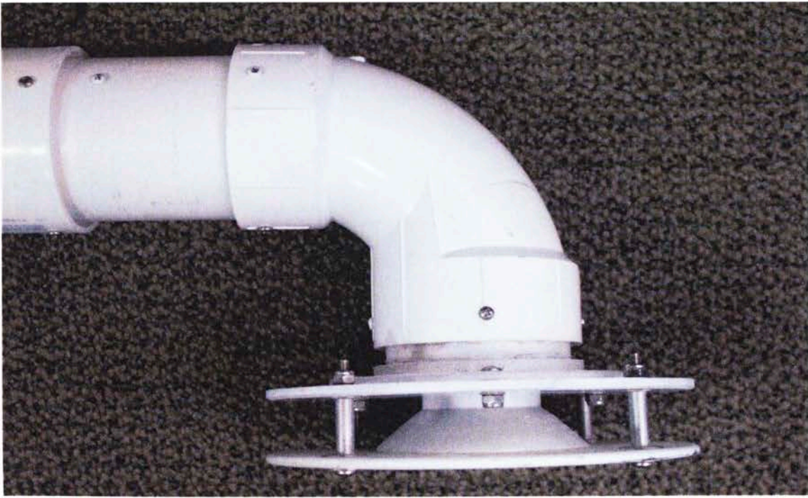
Figure 5: Close up image of the intake section of the U-tube. The intake features two parallel plates as shown and a funnel attached to the lower plate.
