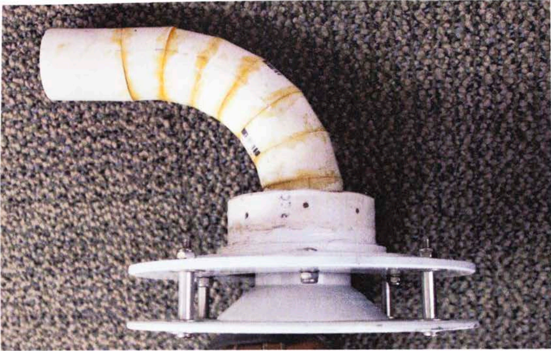
Figure 9: Image depicting the attachment of the inner tube to the funnel on the intake. The inner tube curves through the inside of the Elbow piece, which has been removed for the purposes of this picture.
