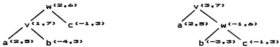
Figure 18. The effect of rotation on the values of dcost and dmin of the vertices. The above is a single right rotation in a solid tree. Values in brackets are (dcost, dmin). Subtrees and dashed edges are skipped for clarity.
