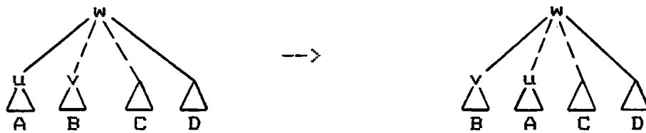
Figure 10. Splicing operation. Node v becomes a left child of w .
