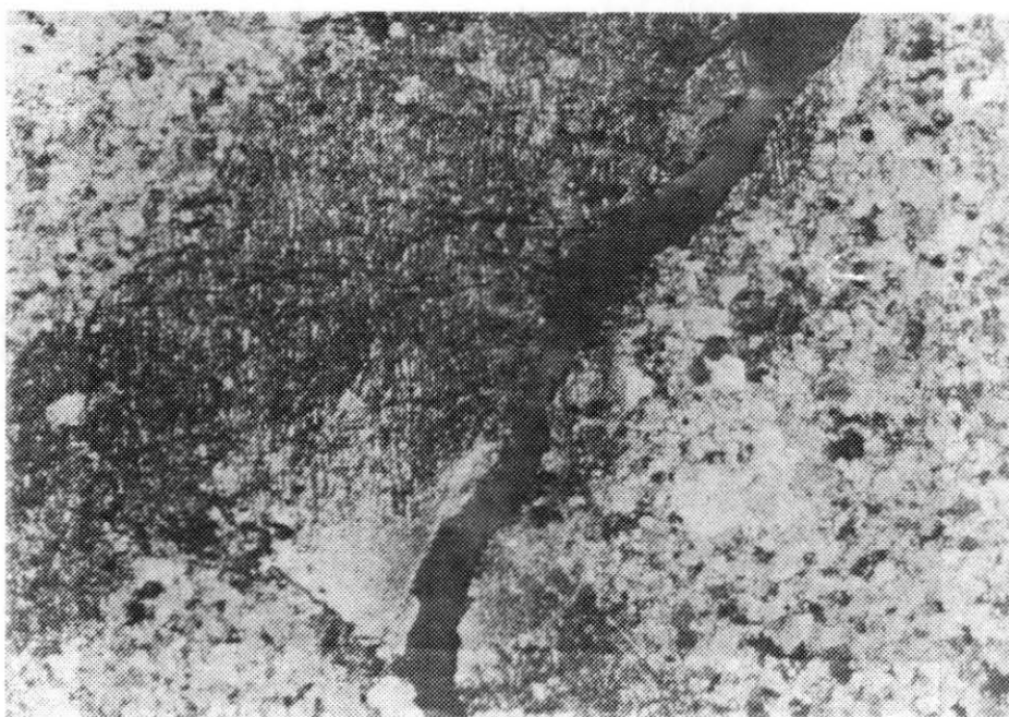
Figure 39. x40 Crossed Nicols. Fracture Porosity, Siliceous Carbonate and Calcite Cements
