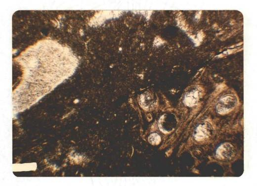
Fig. 16.-Photomicrograph of sparry, crinoid, bryozoan calcilutite. Thin section 2-S-9636, bar approx. 200 µ, plane light, Sinclair, #1 Smith, C NE SE Sec. 29-16N-16W, 9636 ft.
