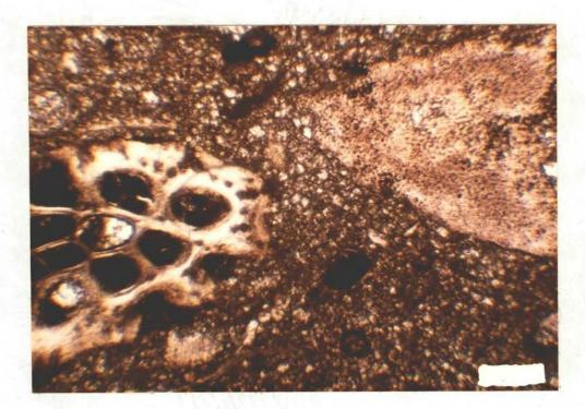
Fig. 10.-Photomicrograph of crinoid stem, bryozoan calcilutite. Crinoid fragment, bryozoan, and pyrite in a microsparite matrix. Thin section 13-R-9716, bar approx. 200 μ, plane light, Sunray, #1 Richardson, SE NW Sec. 19-16N-16W, 9716 ft.
