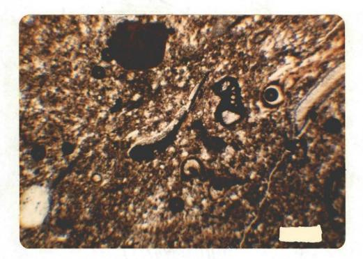
Fig. 9.-Photomicrograph of pyrite and phosphate with fossil fragments in a silty clay matrix. Brown pebble and bands are phosphate, black is pyrite which replaced most of the fossil material. Thin section 1-R-9718, bar approx. 200 μ, plane light, Sunray, #1 Richardson, SE NW Sec. 19-16N-16W, 9718 ft. Fig. 10 shows this rock type in thin section. This lower part is generally tight and non-productive.
