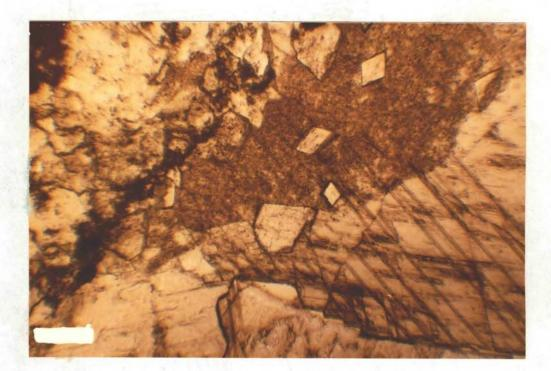
Fig. 12.-Photomicrograph of recrystallized, dolomitized, algal, bryozoan, crinoid calcilutite. Dolomite rhombs in a recrystallized crinoid fragment. Thin section 15-R-9712, bar approx. 200 μ, plane light, Sunray, #1 Richardson, SE NW Sec. 19-16N-16W, 9712 ft. Porosity is developed in this interval as vugs and fractures. Stylolites, vugs, and both filled and open fractures can be seen in thin section (Fig. 13 and 14).
