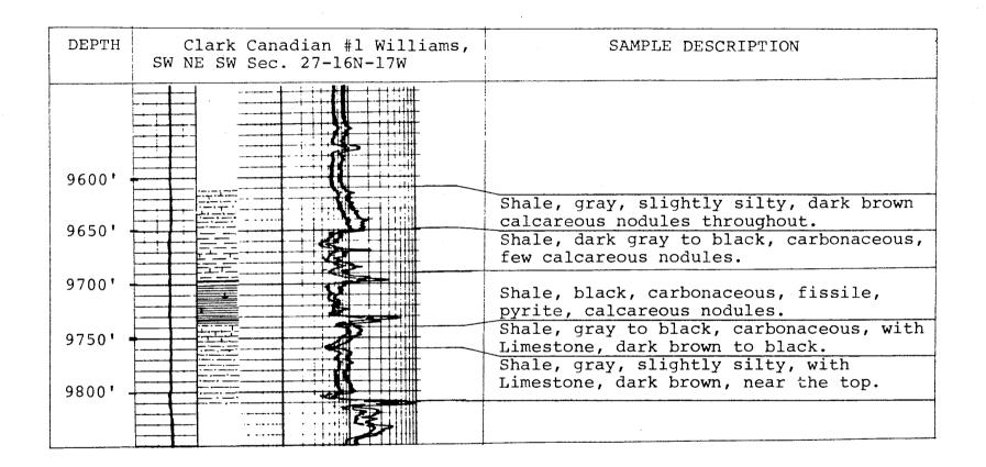
Fig. 17.-Sample description of the "Oswego" in the Clark Canadian, #1 Williams, SW NE SW Sec. 27-16N-17W. The Top "Oswego" Marker is at 9697' and the Base "Oswego" Marker is at 9735', the carbonaceous shale between these is the basin facies of the shelf and bank "Oswego" limestone.
