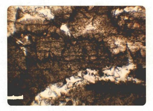
Fig. 13.-Photomicrograph of stylolite. Recrystallized, sparry, pellet, algal calcilutite. Thin section 5-S-8689, bar approx. 200 μ, plane light, Sinclair, #1 Smith, C NE SE Sec. 29-16N-16W, 9689 ft.
