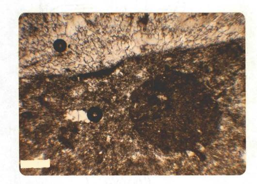
Fig. 11.-Photomicrograph of sparry, algal, pellet calcilutite. Recrystallized algal blade and micritic pellet in calcilutite matrix. Thin section 18-R-9706, bar approx. 200 µ, plane light, Sunray, #1 Richardson, SE NW Sec. 19-16N-16W, 9706 ft.
