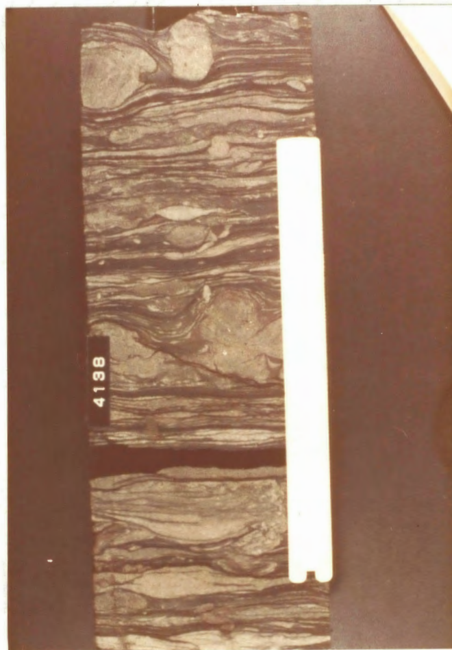
Fig. 18.-Flowage and possibly burrowing in interlaminated sandstone and shale; from Hall-Jones Limited, Sikes No. 3, depth 4133 ft
