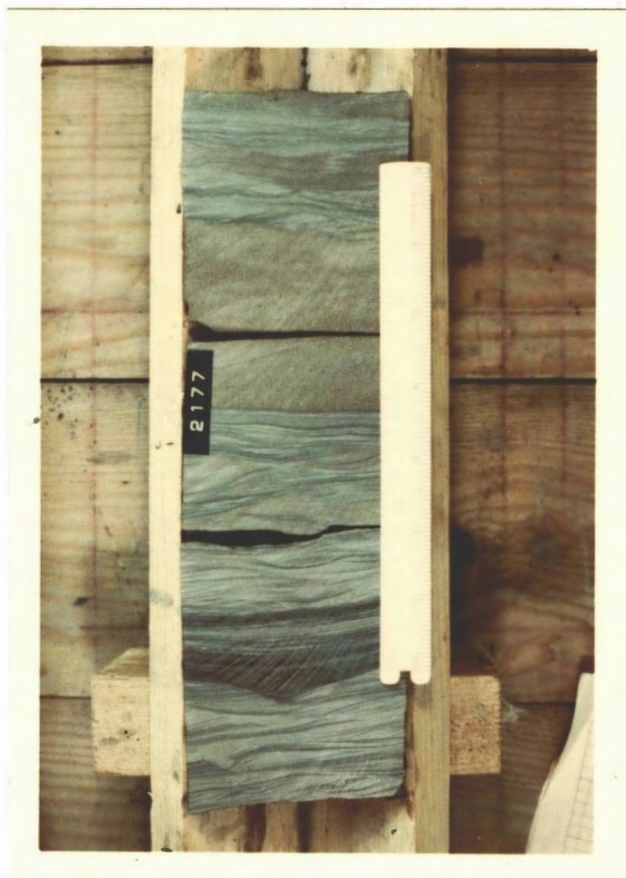
Fig. 15.-Interlamination, small-scale cross-bedding, and minor flowage; from Mack Oil Co., Beaver Creek Unit Tract No. 3, depth 2177 ft
