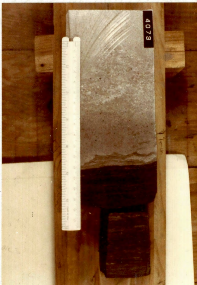
Fig. 20.-Sharp contact between underlying black shale (unit 1) and calcarenaceous sandstone (unit 2); from Pan American Petroleum, Inc., Philpott No. 1, depth 4073 ft
