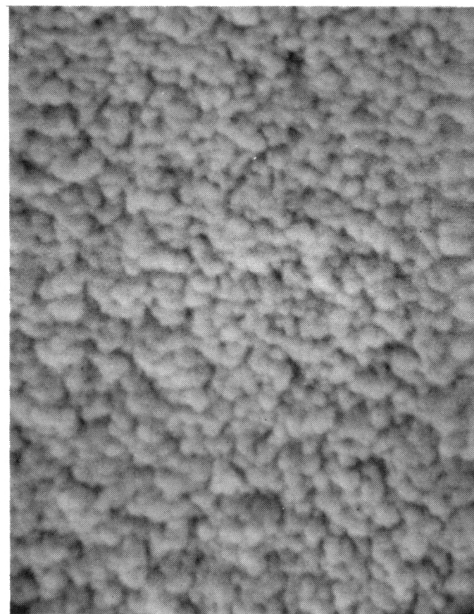
Figure 42. Electron Scan Micrograph for Synthesized CPG-8HO x Resin With Particle Diameter of 125-177 \mu and Pore Size of 544 Å. The Magnification is 100X (Left) and is 30000X (Right)
