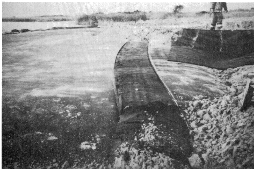
Figure 63. Fabric Seam Field-sewn with Improper Thread Caused Failure to Occur Before Thread Was Replaced with Proper Type
