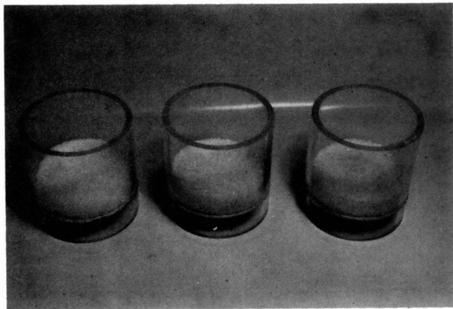
Figure 1. Dust Free and Dust Mixed Samples of Silica Gel in 90 mm Diameter Plexiglass Aeration Bins
