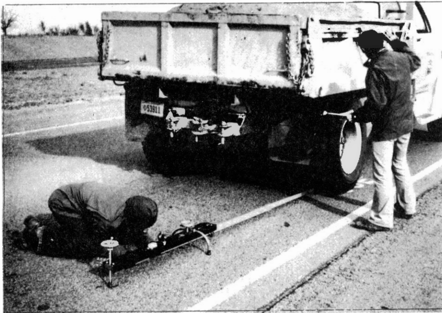
Figure 12. Deflection Measurements with the Benkelman Beam Positioned Normally
