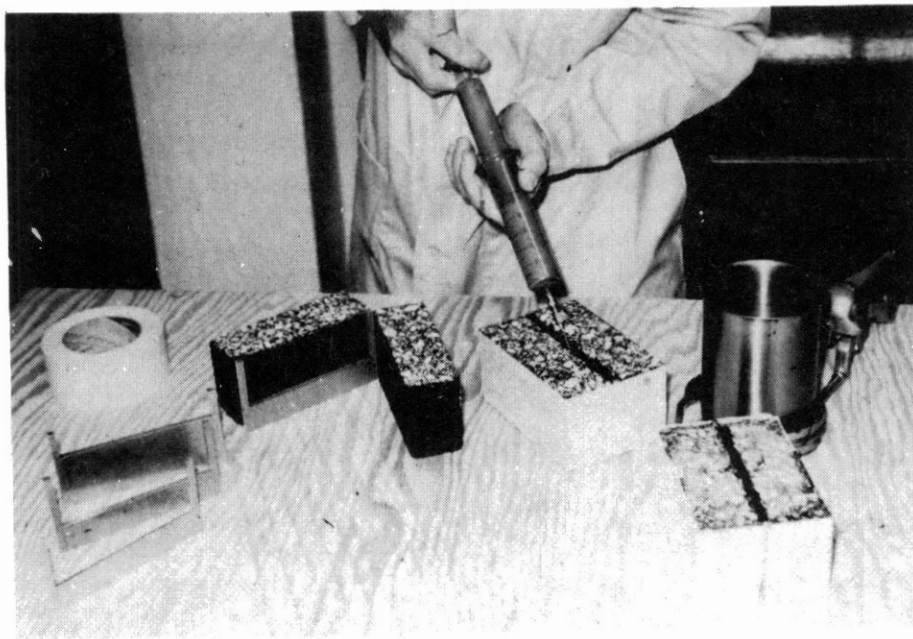
Figure 17. Specimen Preparation for Bond-Ductility Test
