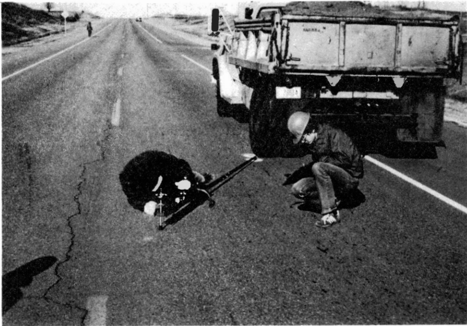
Figure 9. Starting Position For Deflection Measurements
