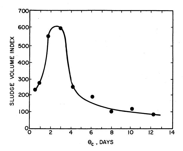
very low or very high solids concentrations, the SVI loses any significance. Busch further reported that while using surface loadings of 150 and 1440 gallons per day per square foot, that although the SVI values were of the same order of magnitude, settling characteristics of the populations were markedly different.
