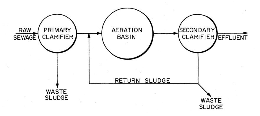
aeration basin and effluent suspended solids. Steady state conditions are attained by wasting that amount of biomass which increases per unit time due to bacterial growth.
