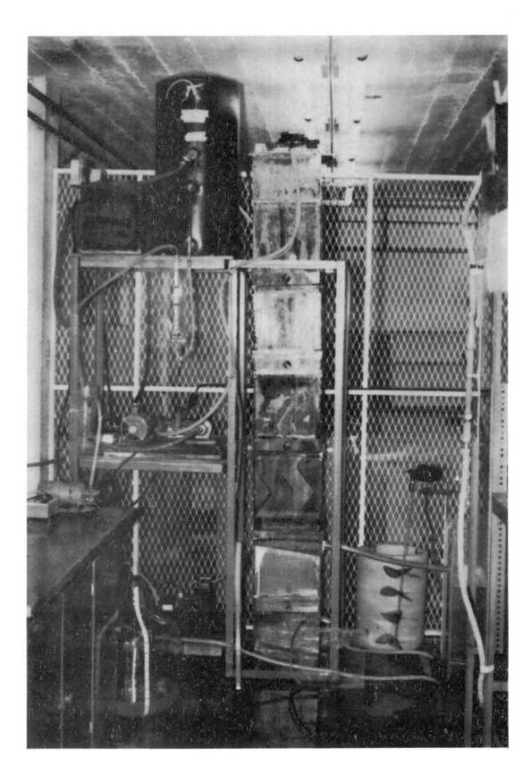
received tap water from a constant head tank. Prior to entering the constant head tank, the water was passed through a coil of copper tubing immersed in a water bath. The temperature of the bath was adjusted such that the water influent to the tower was  $20^{\circ}C \pm 1^{\circ}$ . After passing through the rotameter, the flow was discharged into a wet well where mixing with a concentrated, synthetic waste occurred.
