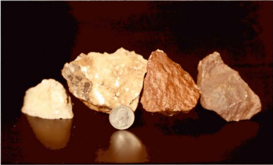
Figure 30. Photograph showing typical surface colors expressed at Red Mountain. X-ray diffraction patterns reveal the yellowish orange coatings to consist of pale yellow jarosite (far left) with sufficient amounts of reddish brown goethite (far right) to provide the respective color.
