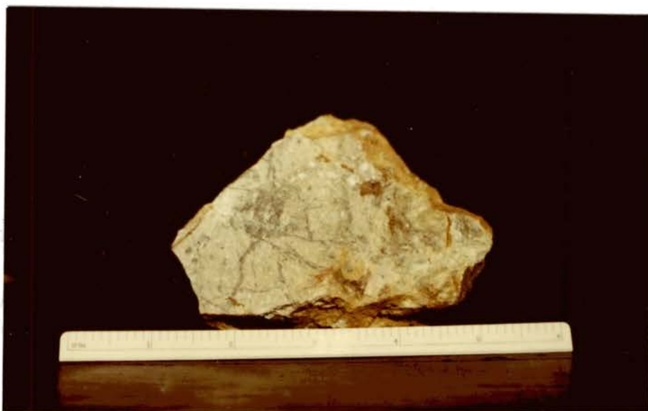
Figure 19. Photograph displaying a lenticular "pod" shaped quartz vein with thin veinlets of quartz radiating outward. Note island of wall rock within pod, crosscutting and displacing relationship of thin veinlets, and fresh pyrite. Close inspection reveals a thin pyrite veinlet at far left in which pyrite is partly replaced by limonitic minerals.
