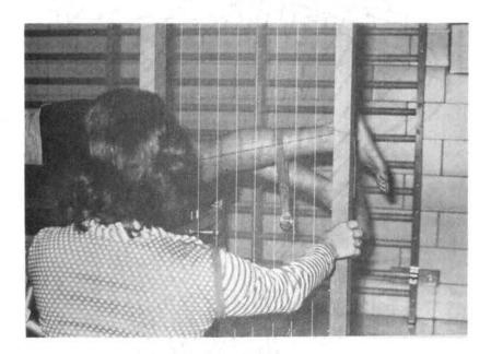
Figure 4. Portable Posture Grid Being Used to Determine a 165 Degree Angle of Extension
