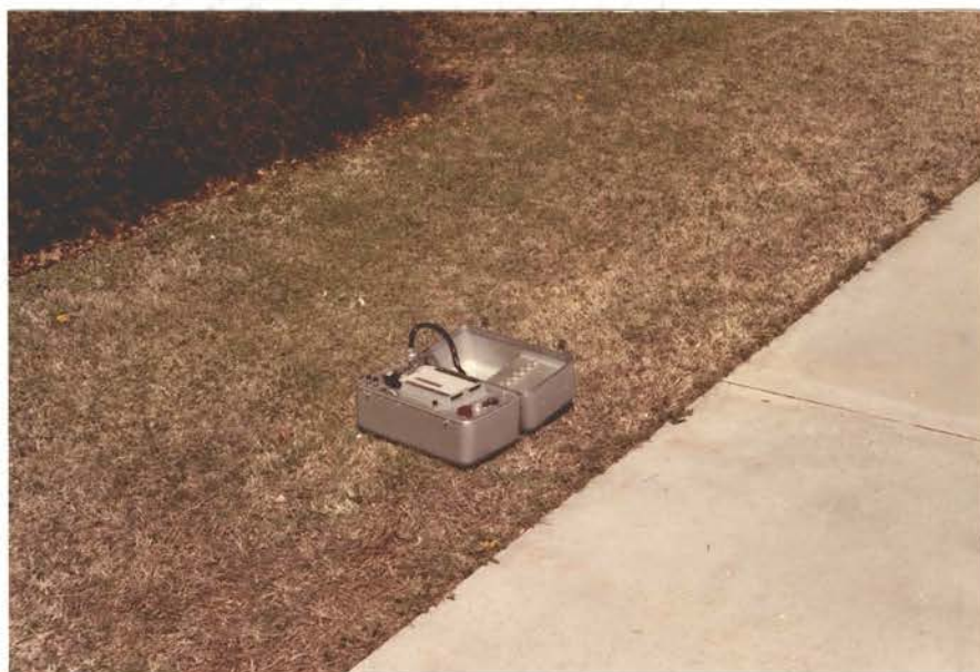
Figure 16. The Electro-Tech Model ER-75-12 portable seismic-refraction unit
