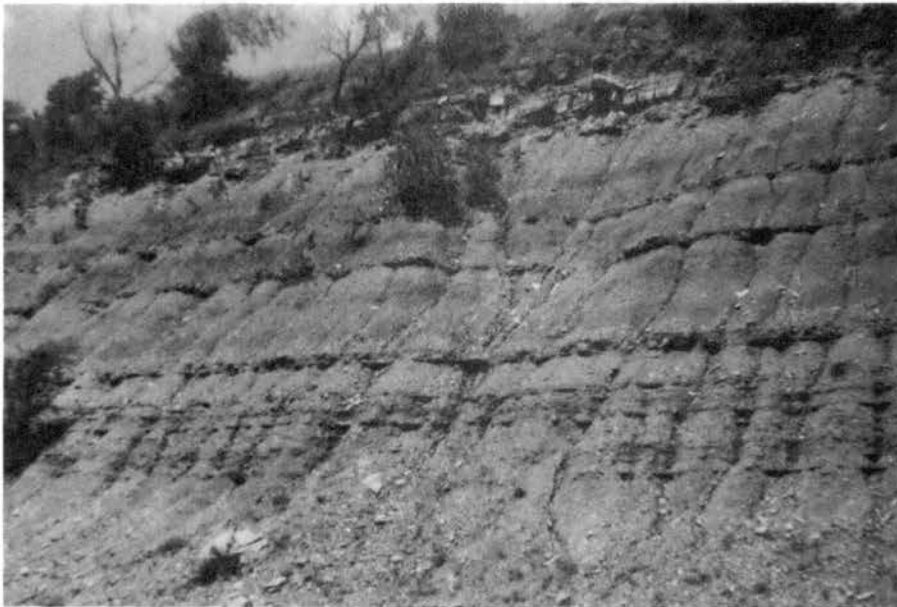
Fig. 9.-Lower marker on outcrop in Sec. 4, T21N, R8E. The marker is a series of interbedded sandstones and shales.
