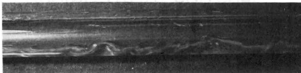
Figure 19. Horizontal Pipe, Wavy Flow
