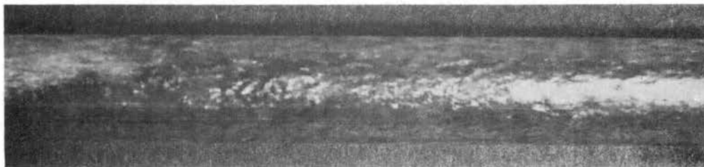
Figure 20. Horizontal Pipe, Annular Flow
