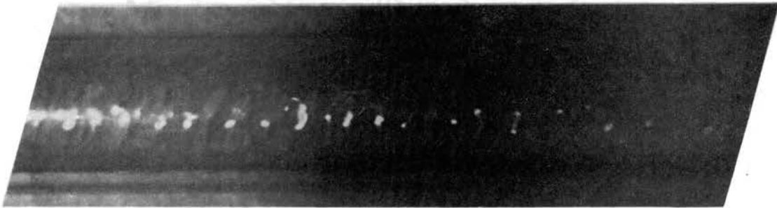
Figure 25. Pipe Inclined 15^\circ , Annular Flow
