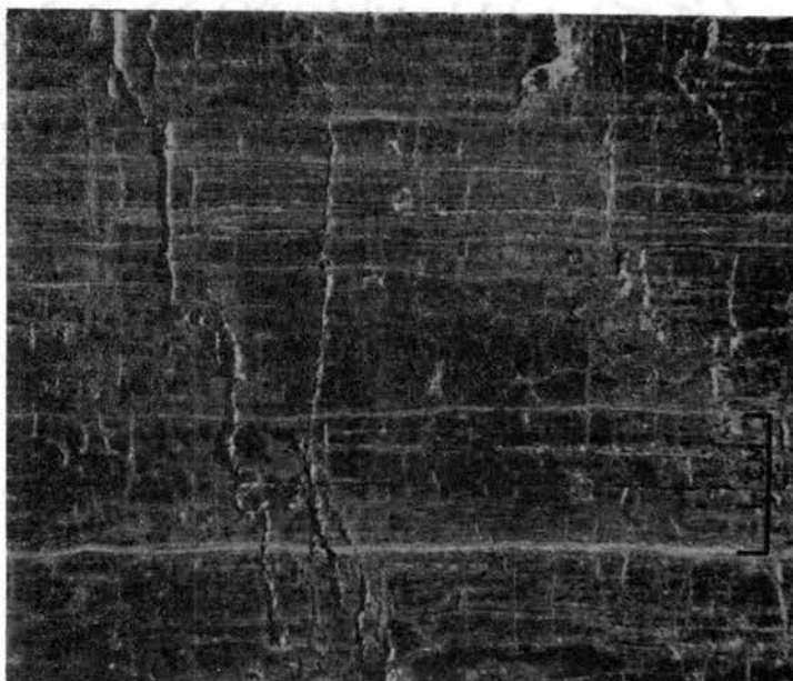
Fig. 18.-Polished section of Stigler coal from Sec. 13, T 11 N, R 19 E, finely-banded to microbanded. Darker banding is vitrain, lighter bands are finely disseminated pyrite bands within bands of attritus and vitrain.
