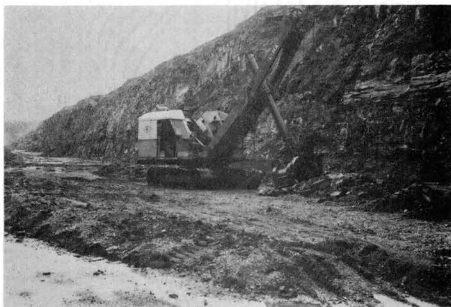
Fig. 26.-Diesel-powered shovel used for loading coal into trucks at the Garland mining operation in Haskell County
