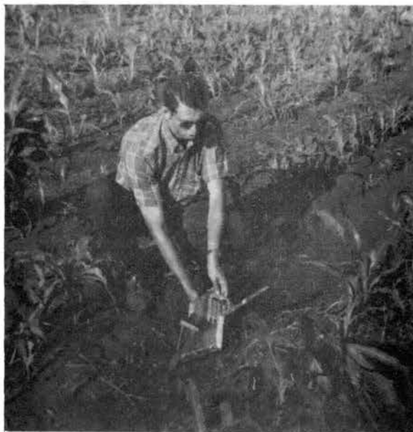
Figure 16. HS Flume Used to Measure the Quantity of Water Flowing Past a Station
