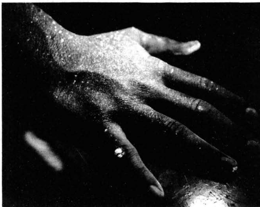
Fig. 18. Accumulation of spray particles on the right hand of the operator while using nozzle 800067 at 2.5 FPS (10 ft/4 sec) at 40 psi.
