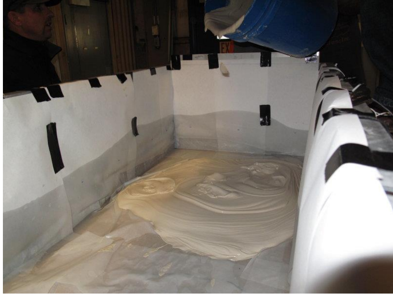
Figure 3-16. Gentle Pouring of Soft Clay on Filter Papers
