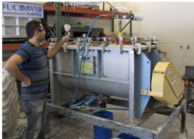
Figure 3-15. Soil Mixer used for Preparing Soft Clay
