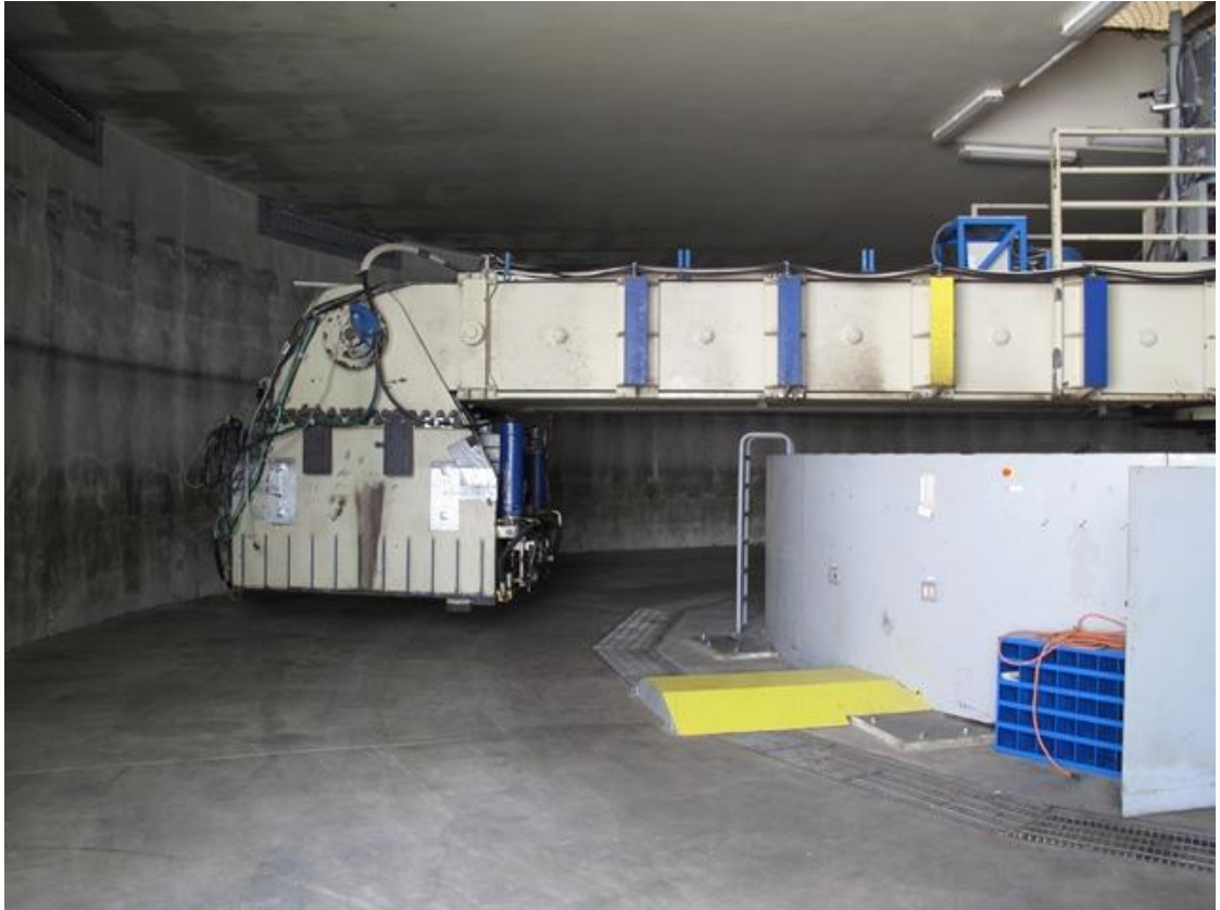
Figure 3-1. The 9-m radius Centrifuge at the Center for Geotechnical Modeling (CGM) at University of California, Davis (UC Davis)
