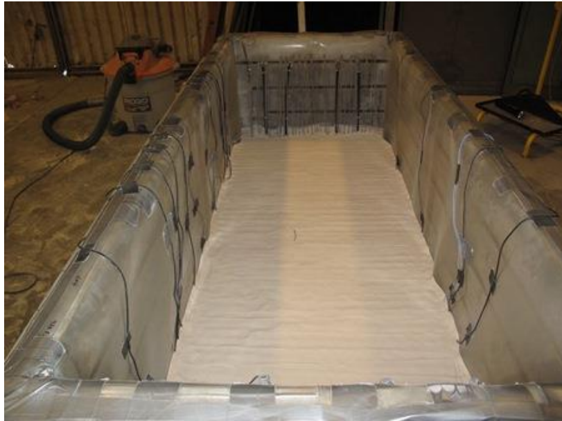
Figure 3-12. Dense Nevada Sand Layer Graded using a Vacuum
