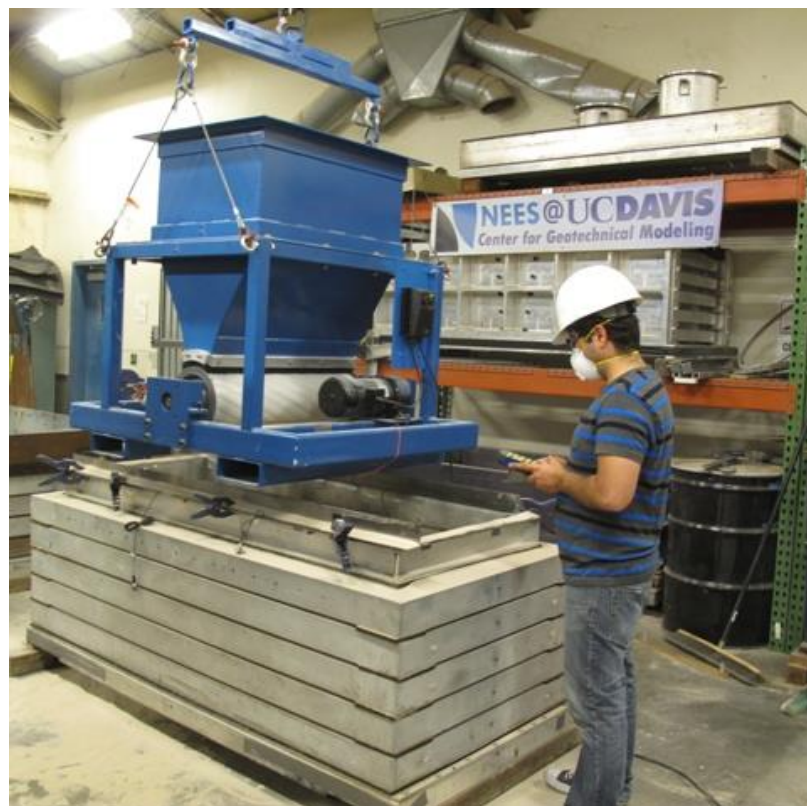
Figure 3-11. Nevada Sand Pluviation
