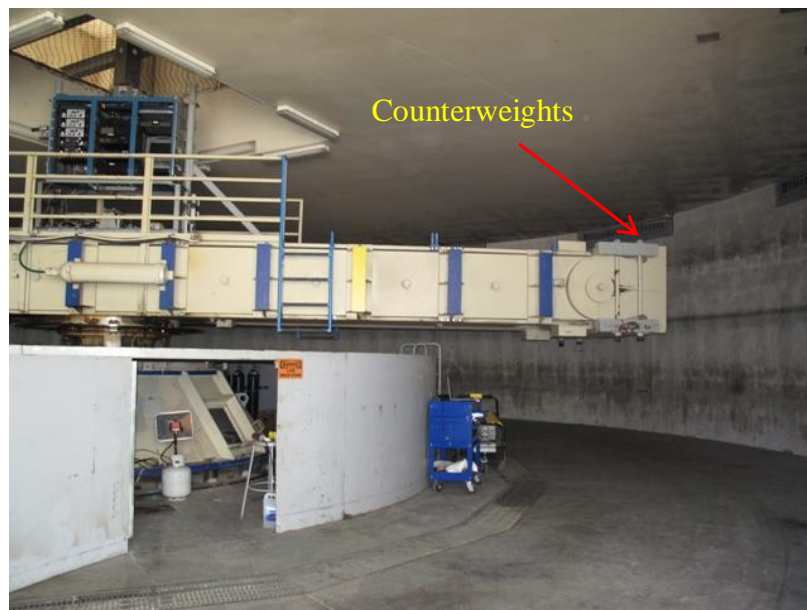
Figure 3-3. Balancing Counterweights on the Centrifuge Arm
