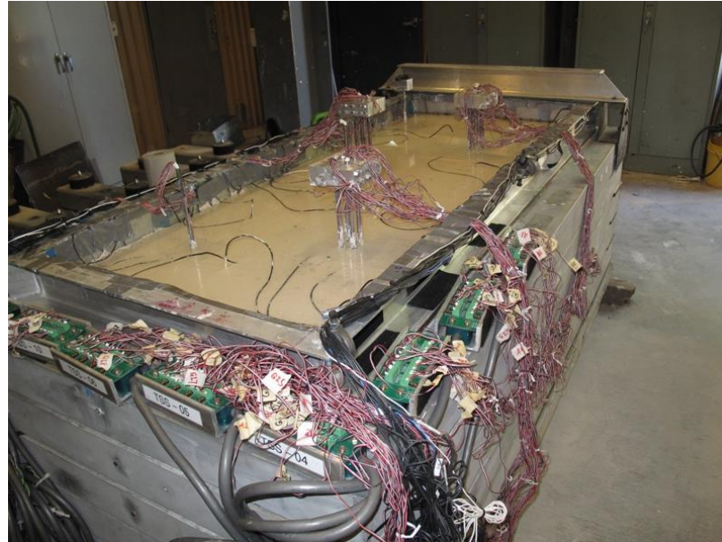
Figure 3-25. Centrifuge Model before Going on the Centrifuge Arm
