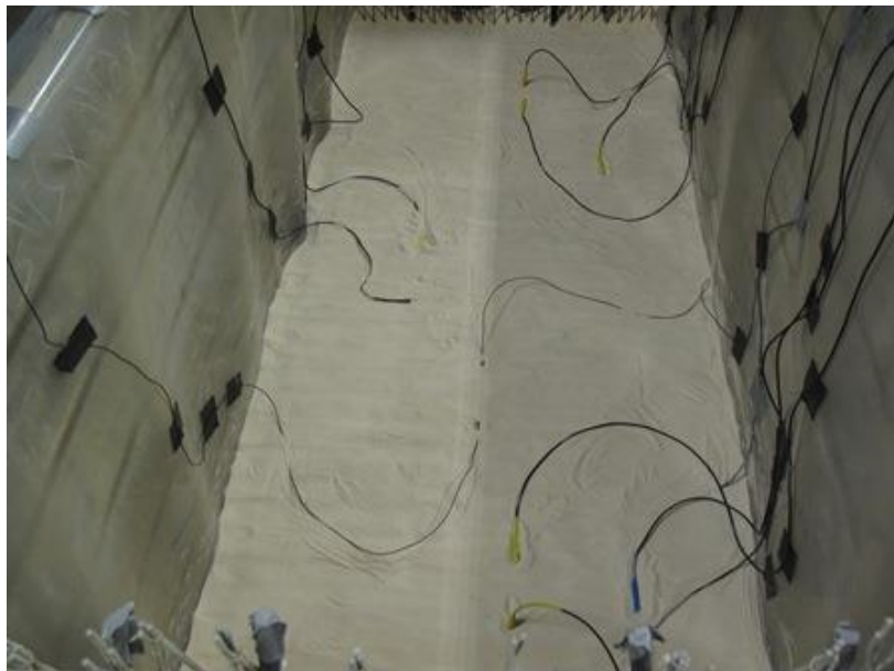
Figure 3-13. Placement of Instruments in Dense Nevada Sand Layer
