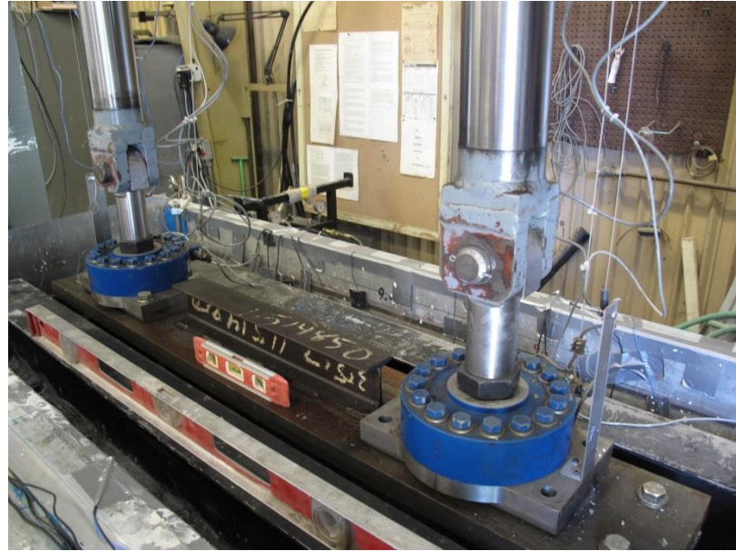
Figure 3-18. Soft Clay Layer under Hydraulic Press
