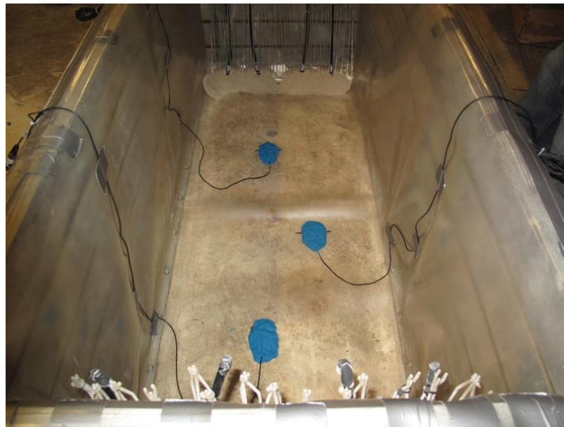
Figure 3-6. Accelerometers at the Bottom of FSB1 Container
