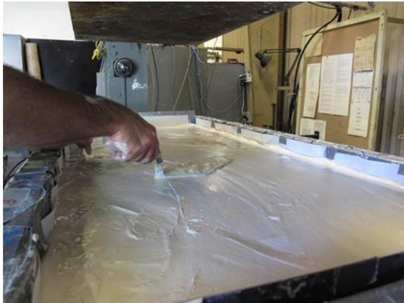
Figure 3-17. Leveling Soft Clay Surface
