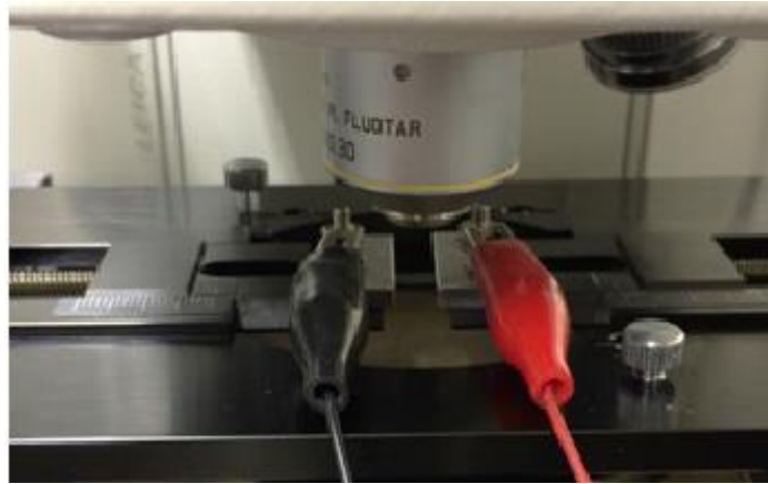
Figure 4.3. Experimental setup used to image the subsurface failure mechanics in CNT composite samples under tensile strain. The composite sample is mounted directly under the objective.
