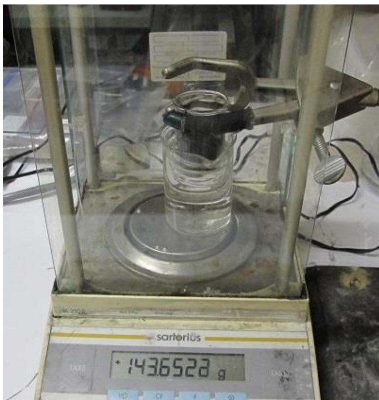
Figure 3.1. The setup used to measure the water absorbed by CB
