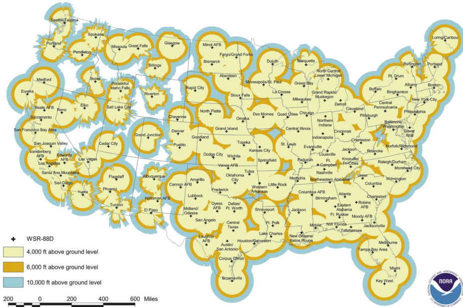
Figure 1.2: Current WSR-88D coverage at 4,000, 6,000, and 10,000 ft above ground level (in yellow, gold, and blue shadings, respectively). Calculations are based on the radar beam height approximation in Doviak and Zrnić (1993), and the image was provided by the National Oceanic and Atmospheric Administration (NOAA).
