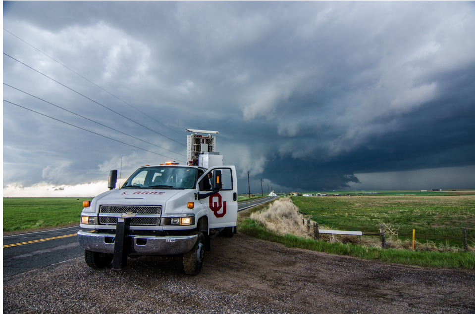
Figure 5.27: The atmospheric imaging radar scanning a tornadic supercell east of Denver, CO on 21 May 2014.
