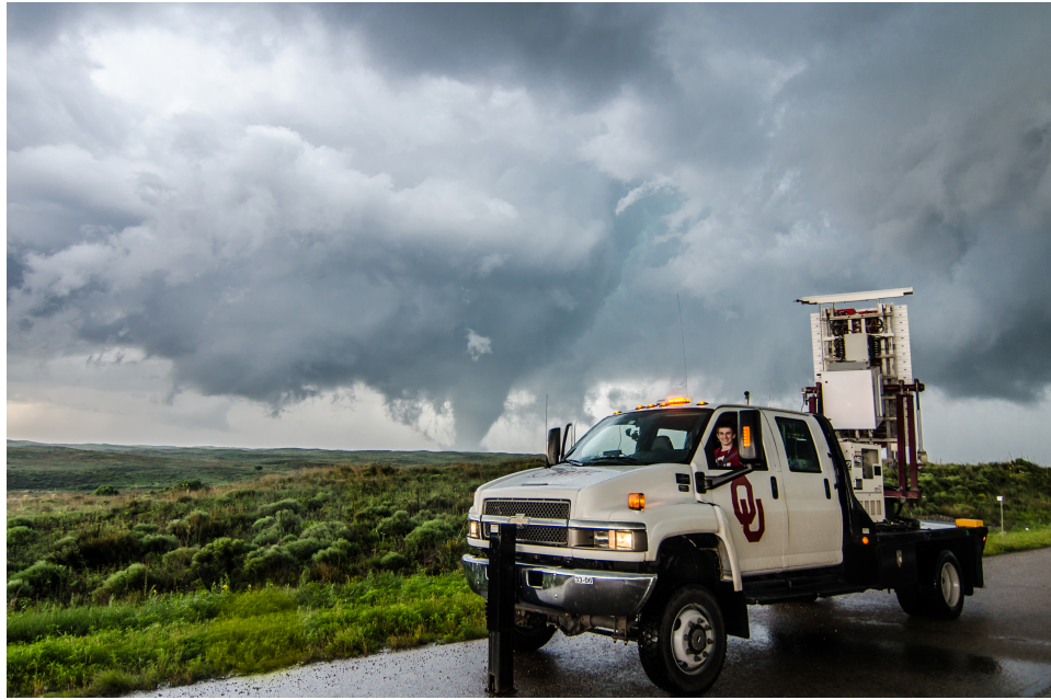
Figure 5.37: The atmospheric imaging radar scanning a tornado north of Canadian, Texas on 27 May 2015.
