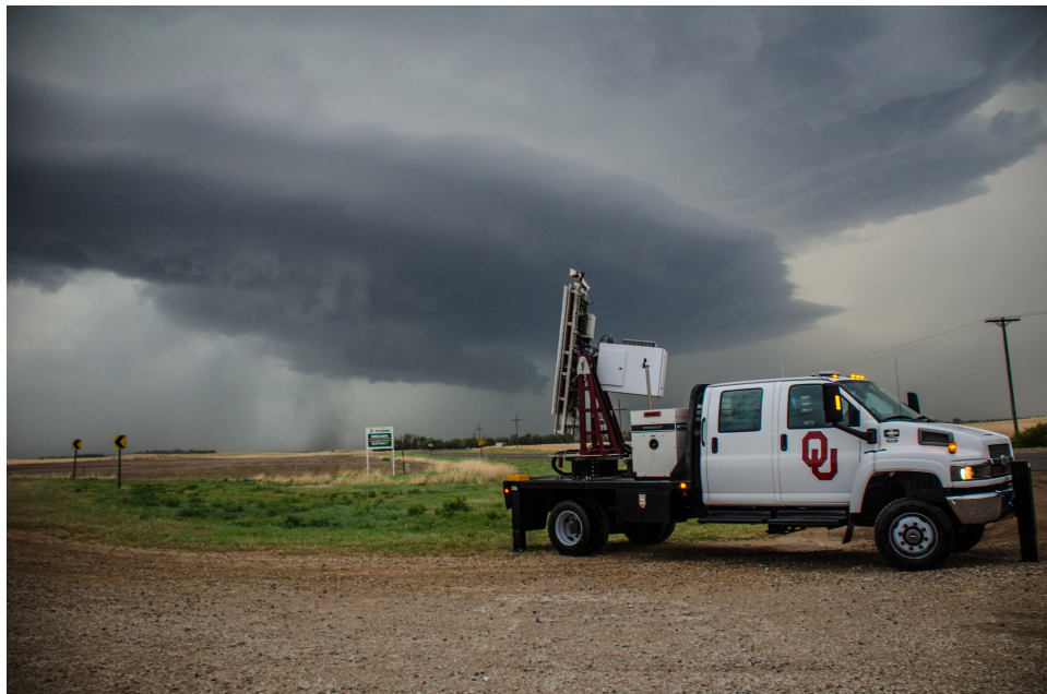
Figure 5.25: The atmospheric imaging radar scanning a landspout tornado south of Great Bend, Kansas on 11 May 2014.
