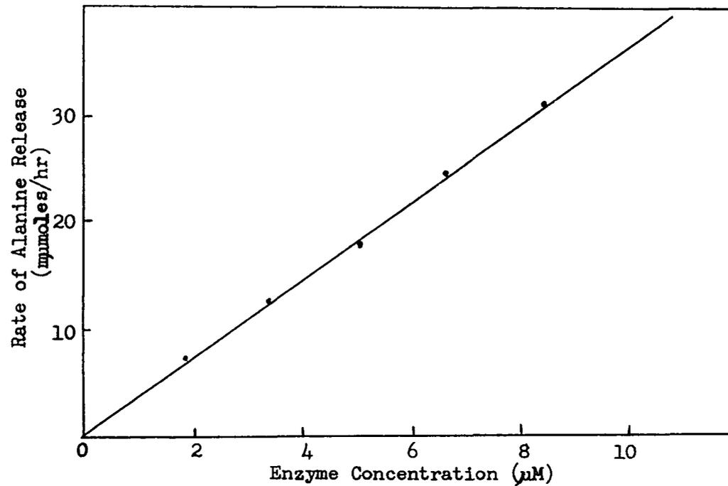
Figure 16. Proportionality of velocity to enzyme concentration in the gastricsin assay. The extent of peptide hydrolysis was determined by amino acid analysis. The substrate was 0.5 mM CBZ-L-tyr-L-ala. Hydrolyses were performed in 0.1 M sodium citrate-HCl buffer, pH 2.0, and 37°.
