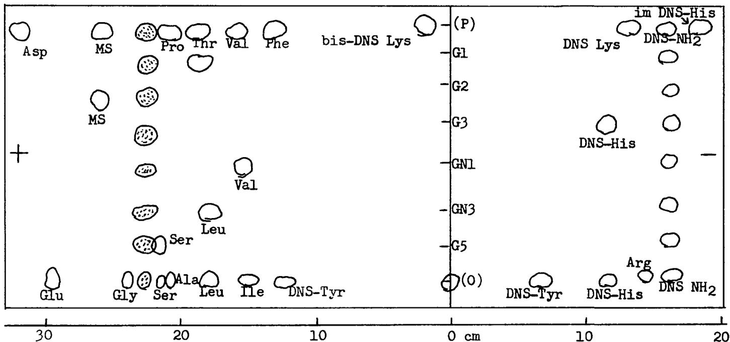
Figure 5. Electrophoresis of DNS-amino acids from the hydrolysis of DNS-derivatives of gastricsin peptides (G1, G2, G3, GN1, GN3, G5) on Whatman No. 3 MM paper at pH 4.55 on a flat plate. ⊕ : blue fluorescence of dansyl sulfonic acid, ○ : yellowish blue fluorescence of DNS-amino acids. (P) and (O) are standard DNS-amino acid mixtures.
