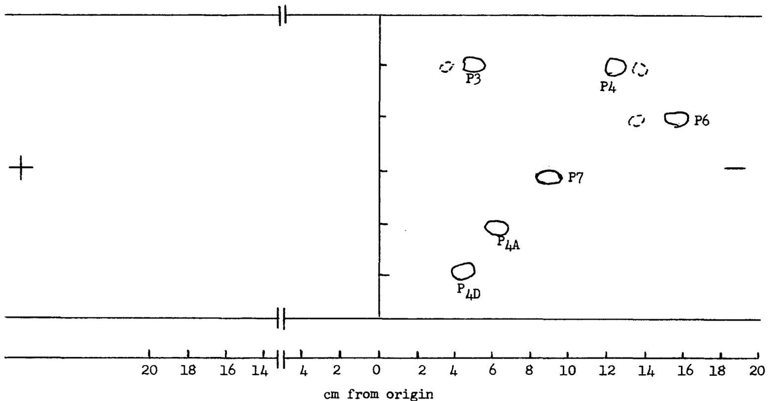
Figure 10. High voltage paper electrophoretic separation of peptides derived from the hydrolysis of oxidized ribonuclease A by pepsin. The electrophoresis was carried out at 4000 volts (80 volts/cm) at pH 3.5 for 100 minutes. The solid circles indicate the major spots, and the dotted circle indicate trace peptides.
