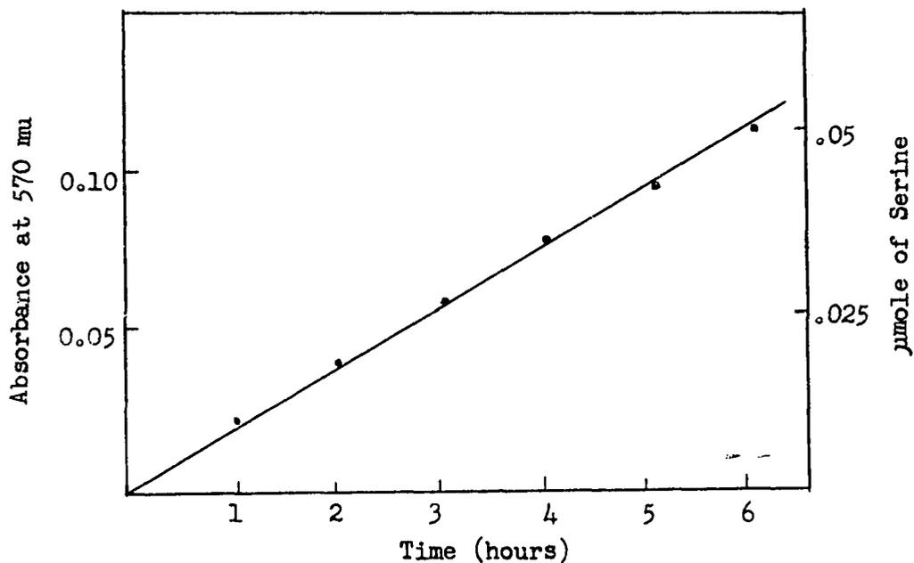
Figure 14. Hydrolysis of N-CBZ-L-tyrosyl-L-serine by gastricsin (0.4 mg) at pH 2 and 37°. The extent of hydrolysis was determined by the ninhydrin method. Aliquots (0.1 ml) were analyzed at one hour intervals.
