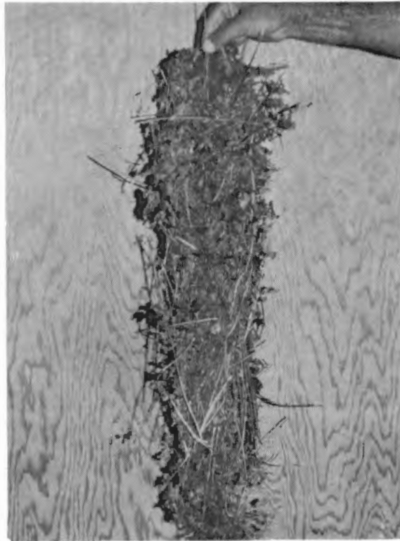
Figure 30. View of Hay Batting Made of Crushed Alfalfa and Orzan After Durability Tests (Supported Vertically by Hand)
