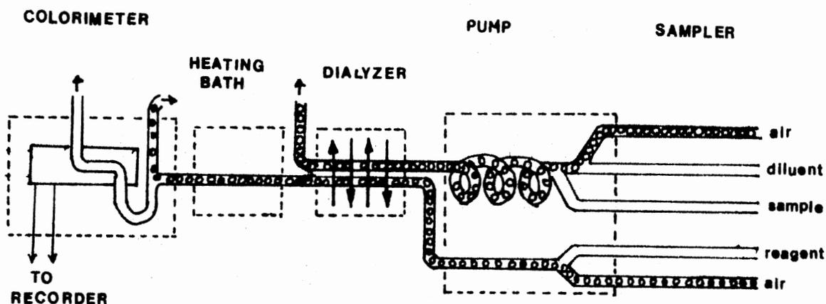
Figure 1. Schematic Representation of the Basic AutoAnalyzer Modules
