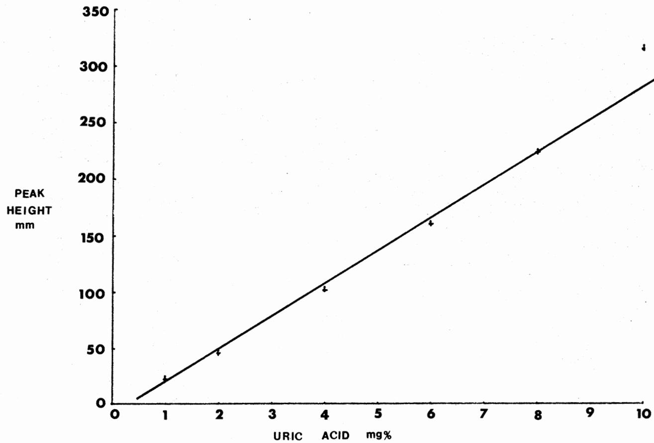
Figure 30. Calibration Curve for Uric Acid Determination
