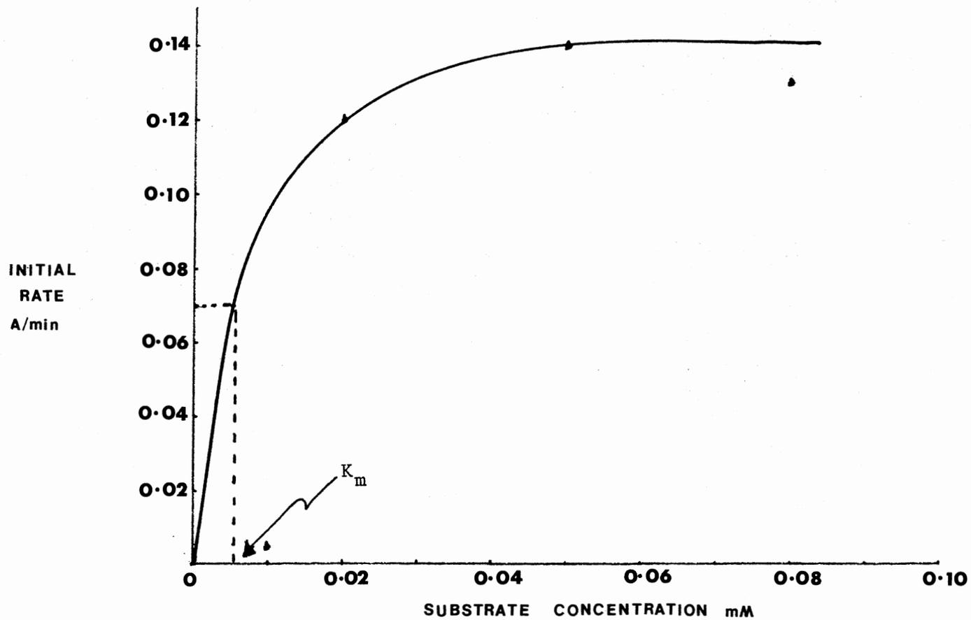
Figure 26. Apparent  $K_m$  Value Determination for Native and Immobilized Uricase
