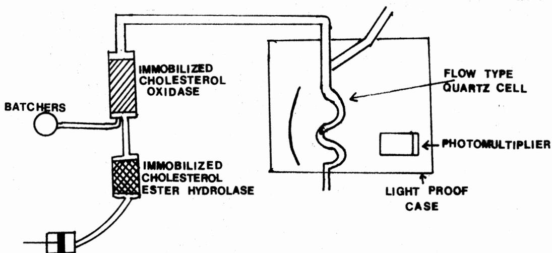
Figure 13. Schematic Diagram of Setup for Treating Sample and Measuring the Chemiluminescence
