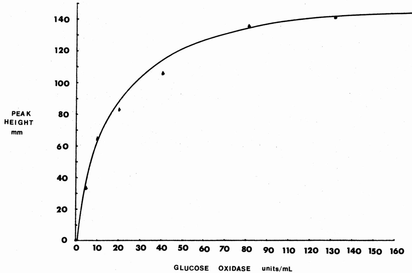
Figure 19. Calibration Curve for Determination of Glucose Oxidase
