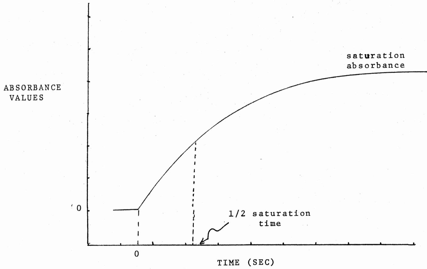
Figure 24. Curve That Defines Terms Used in Discussion the Kinetics of Reactions of Amino Acis
