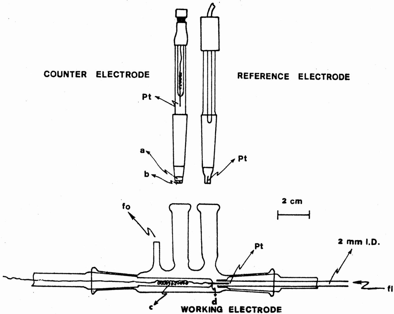
Figure 16. Design of the Amperometric Three Electrode System
