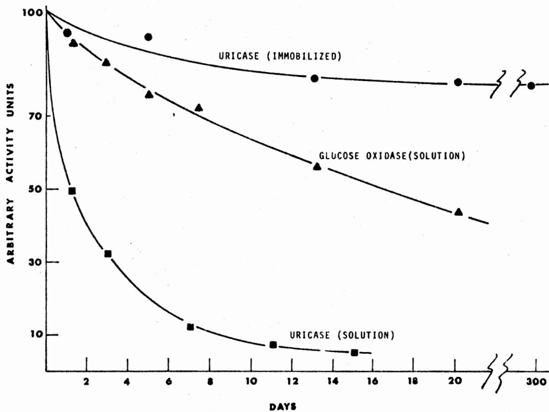
Figure 6. Long-Term Stability of Soluble Glucose Oxidase and Uricase and Covalently Bonded Immobilized Uricase
