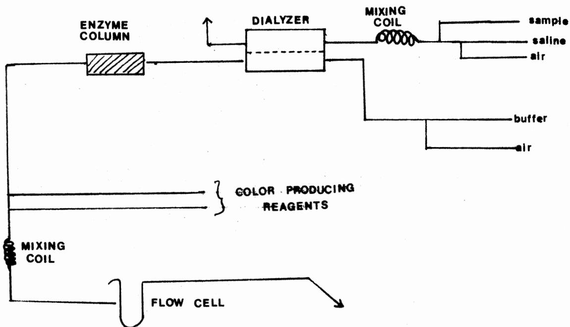
Figure 11. A Simplified Flow Diagram for Spectrophotometric Analysis Using Immobilized Enzyme Column Reactor Integrated Into the AutoAnalyzer I
