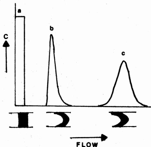
Figure 5. Typical Peak Profiles (a) at Point of Injection (b) Shortly After Injection (c) Long After Injection
