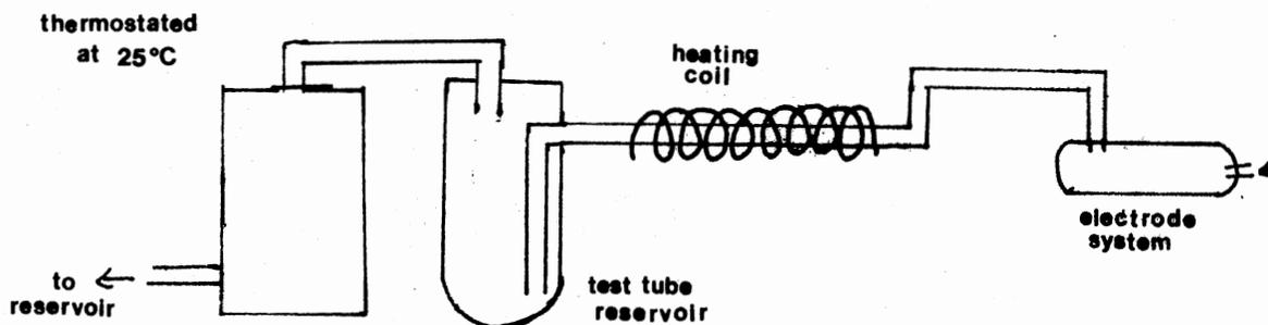
Figure 17. Heating Coil and Other Required Materials for Inactivating Glucose Oxidase
