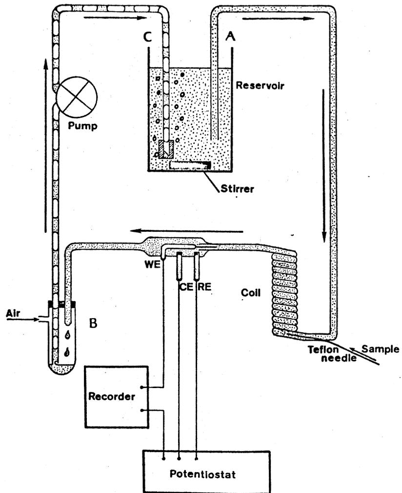
Figure 14. Experimental Setup Used for the Amperometric Determination of Enzymes or Substrates
