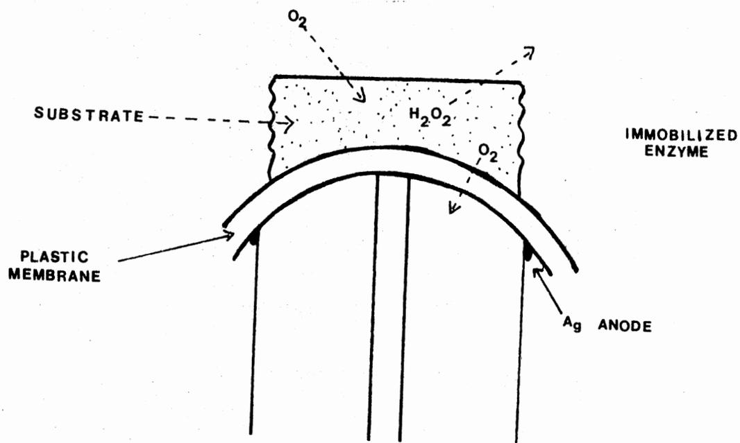
Figure 8. Schematic Diagram of an Enzyme Electrode With Amperometric Sensor
