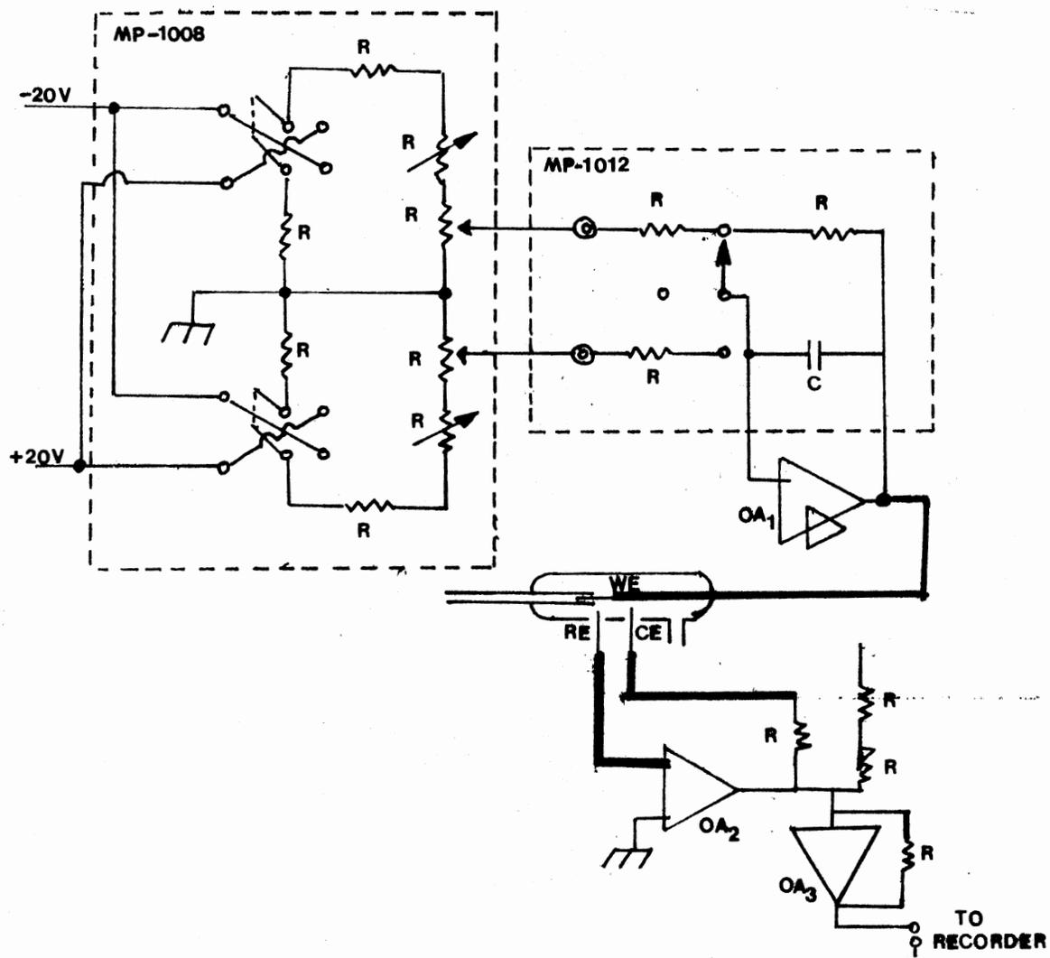
Figure 15. Potentiostat Arrangement for Amperometric Determinations
