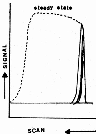
Figure 4. Typical Signals of AutoAnalyzer With Different Concentration Profiles
