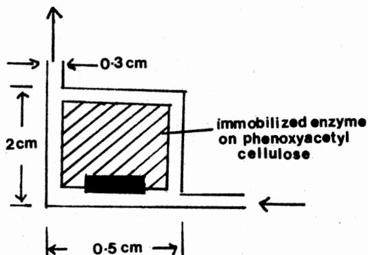
Figure 18. Configuration of Plexiglass Chamber for Containing Immobilized Glucose Oxidase
