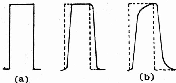
Figure 3. Signals of the AutoAnalyzer (a) Ideal (b) Typical
