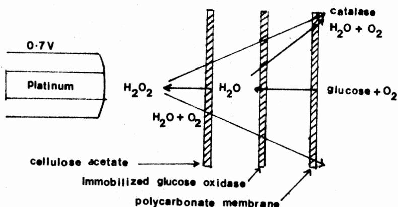
Figure 10. Probe Membrane Combination Used in the Yellow Spring Instrument Company's Glucose Analyzer
