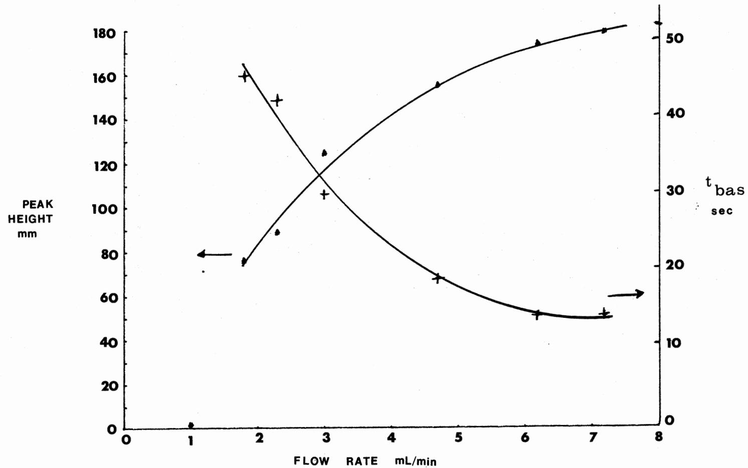
Figure 32. Effect of Flow Rate on Peak Height and on Return to Baseline
