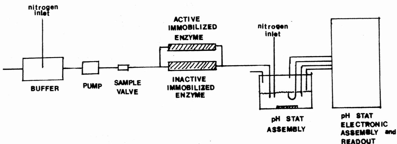
Figure 12. Block Diagram of Flow Coulometric Immobilized Enzyme Analyzers
