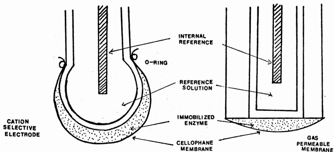
Figure 7. Schematic Diagram of Potentiometric Sensors
