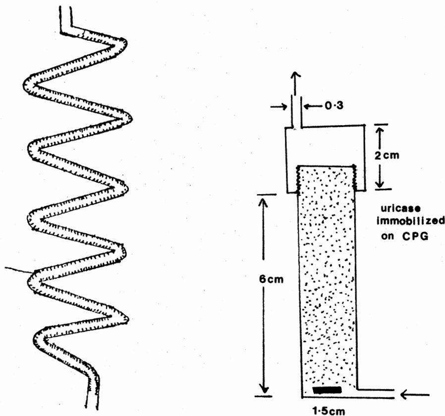
Figure 22. Design of Coil and Slender Chamber
