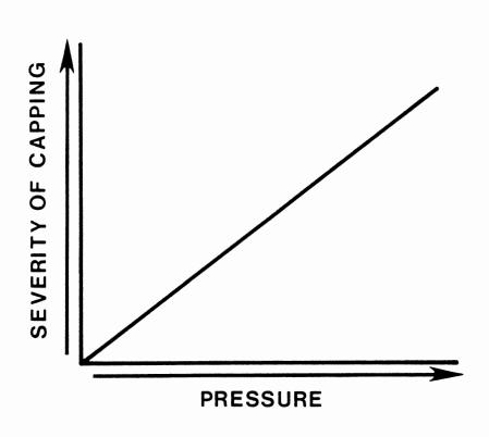
percent of PEG increased. Since PEG is a lubricant, the author felt that its lubricating capabilities caused the sliding of particles instead of cohesion and thus promoted capping.
