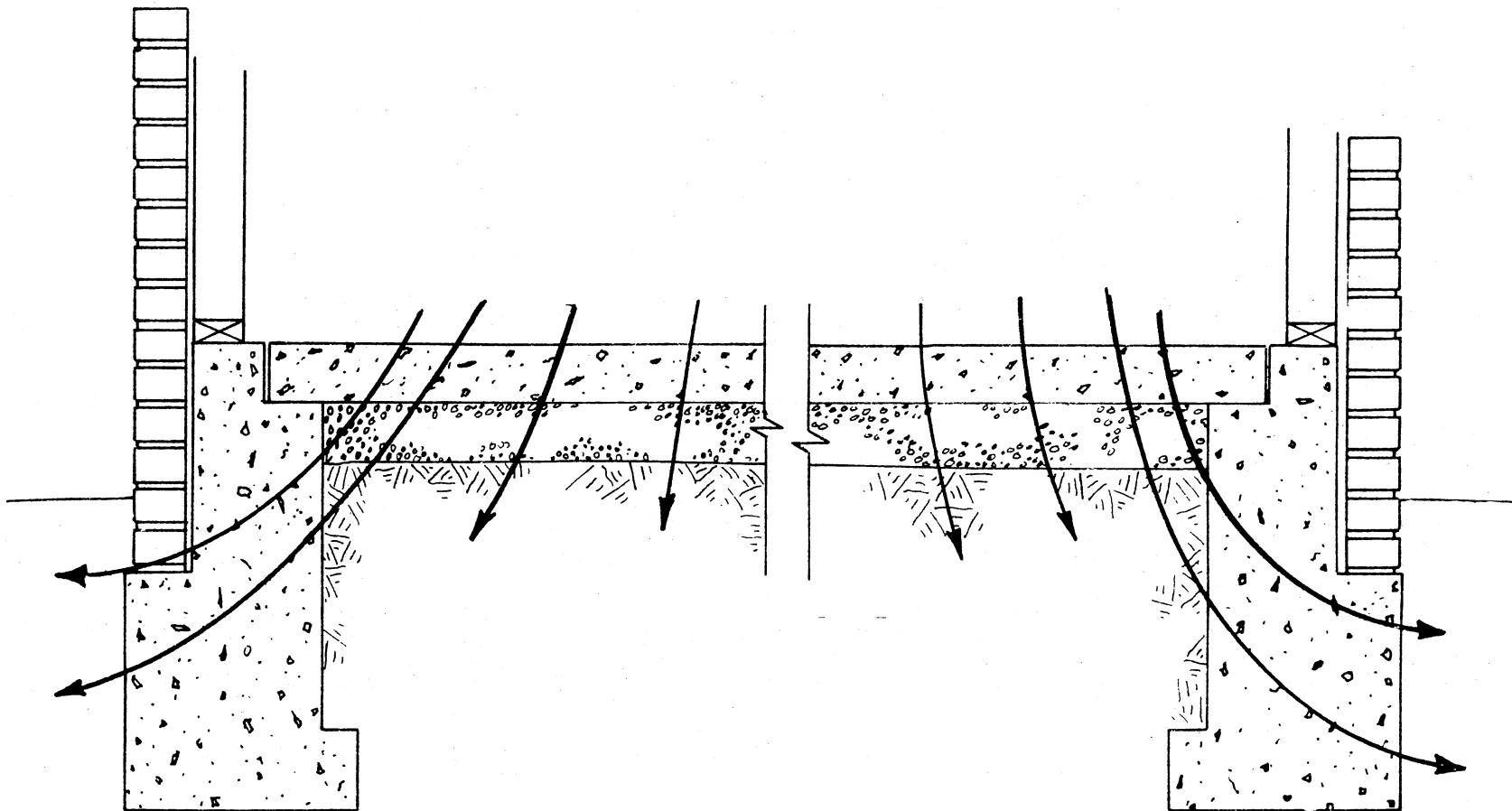
Figure 3. Heat Flow Patterns For Concrete Slab-on-Grade Floors
