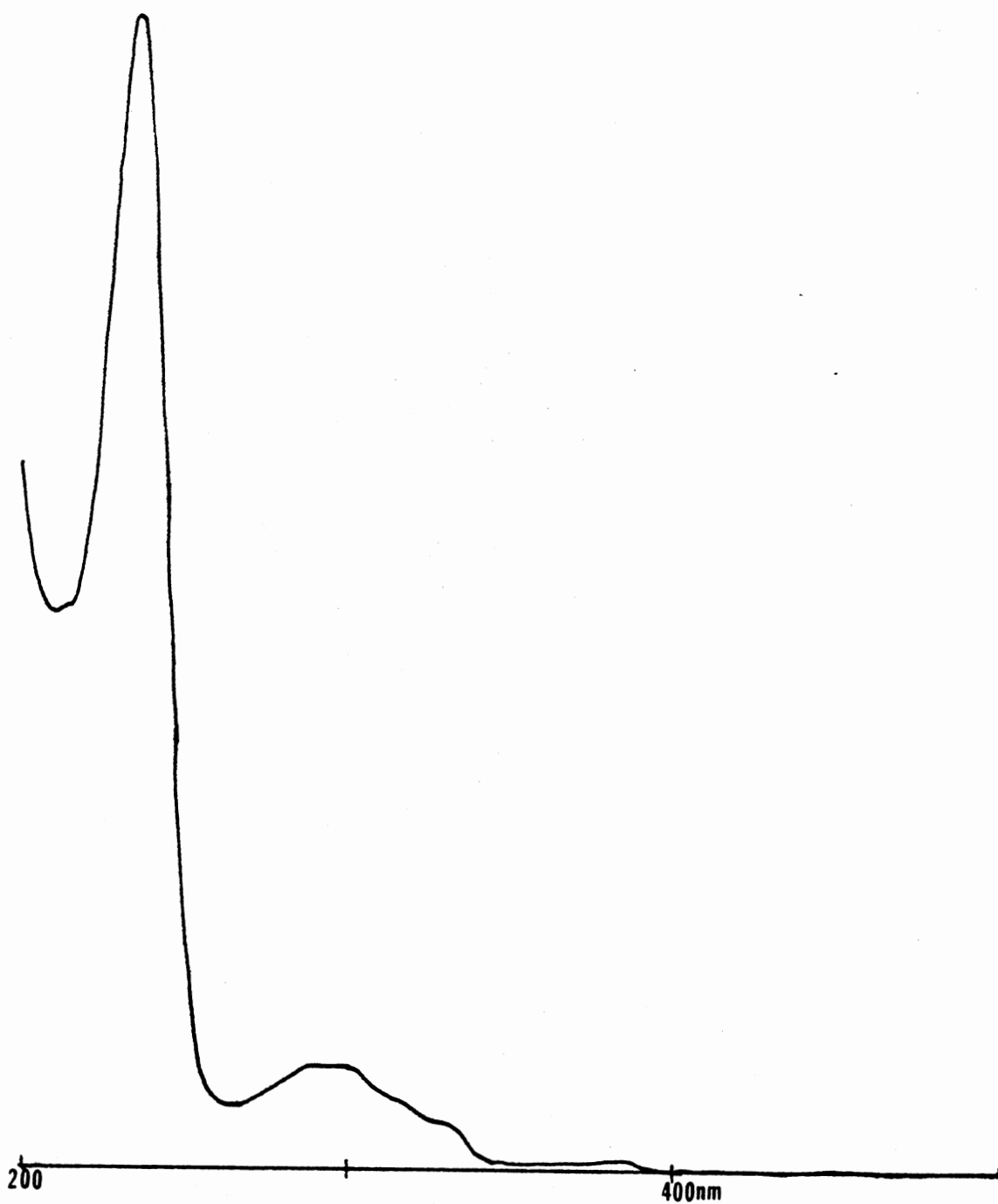
Fig. 1 UV-visible Absorption Spectrum of DHC, 10.3 \mu\text{M} in MOPS Medium; Scanned with MOPS Medium Blank.
