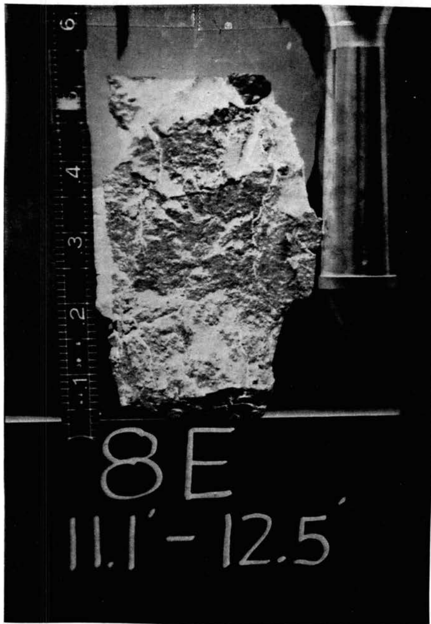
Figure 46. Secondary Clay Structure, Fissures, Sample 8E at Boring W4, Wagoner Site
