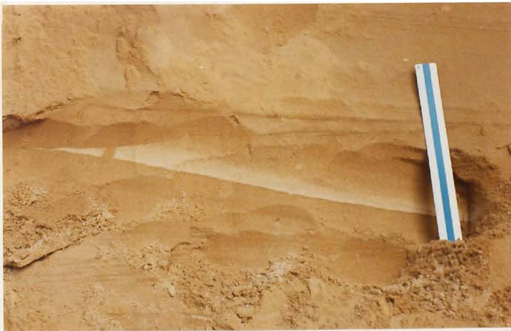
Figure 24. Upward-darkening Unit and the Wedging Effect of Multiple Bounding Surfaces, Deep Cut Site.
