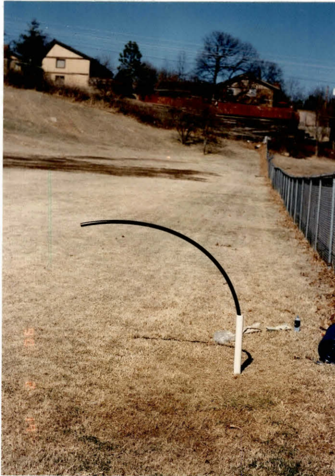
Figure 5. Well I-1 with Inertial Pump Tube
