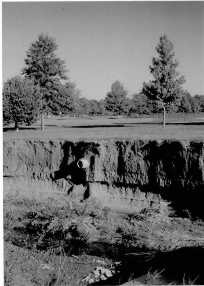
Figure 9. Cut Bank #7 Where Fred Creek Channel Exposes Mollic Soil of Flood Plain
