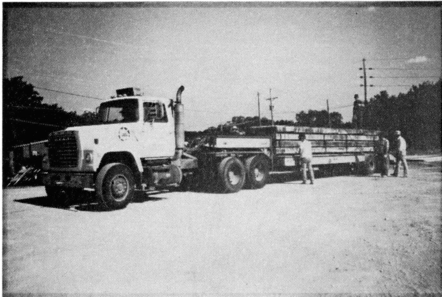
Figure 29. Four Panels on Flatbed Trailer Ready for Transport
