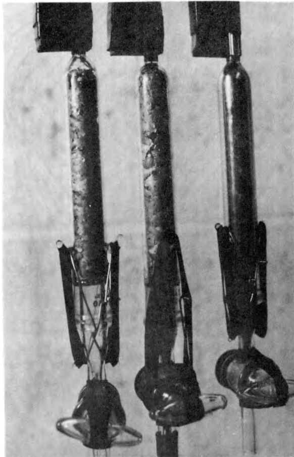
Figure 8. Dilatometers Filled with Peanut Skins (Dilatometer on the Right also Contains Mercury.)
