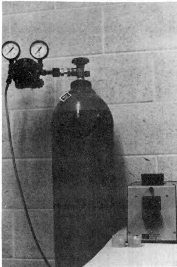
Figure 4. Helium-Air Comparison Pycnometer and Helium Cylinder with Pressure Regulator
