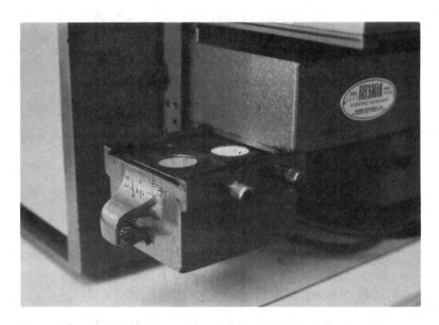
Figure 23. Sample Drawer of the Reflectance Attachment.
