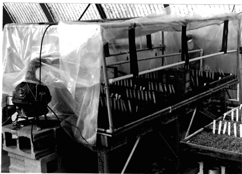
Fig. 5. Mist chamber used for the pathogenicity studies.
