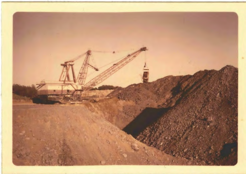
Figure 1. Dragline Near Stigler, Oklahoma Removing Over 90 Feet of Overburden for an 18 Inch Seam of Coal.
