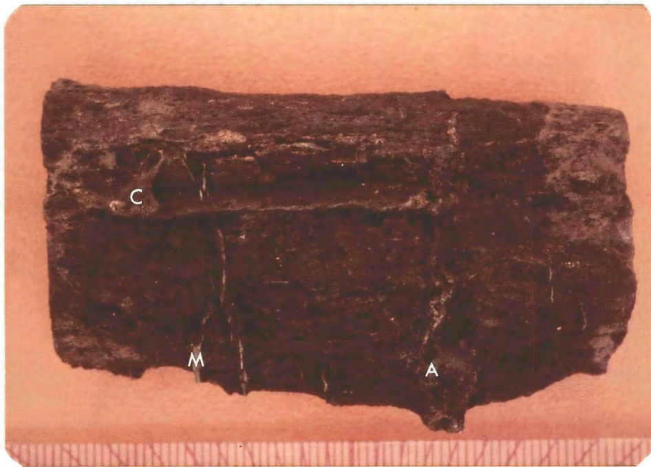
Fig. 6.-Replacement of carbonaceous wood by chalcocite (C), malachite (M), and azurite (A). From channel deposit in Sec. 23, T20N, R3E
