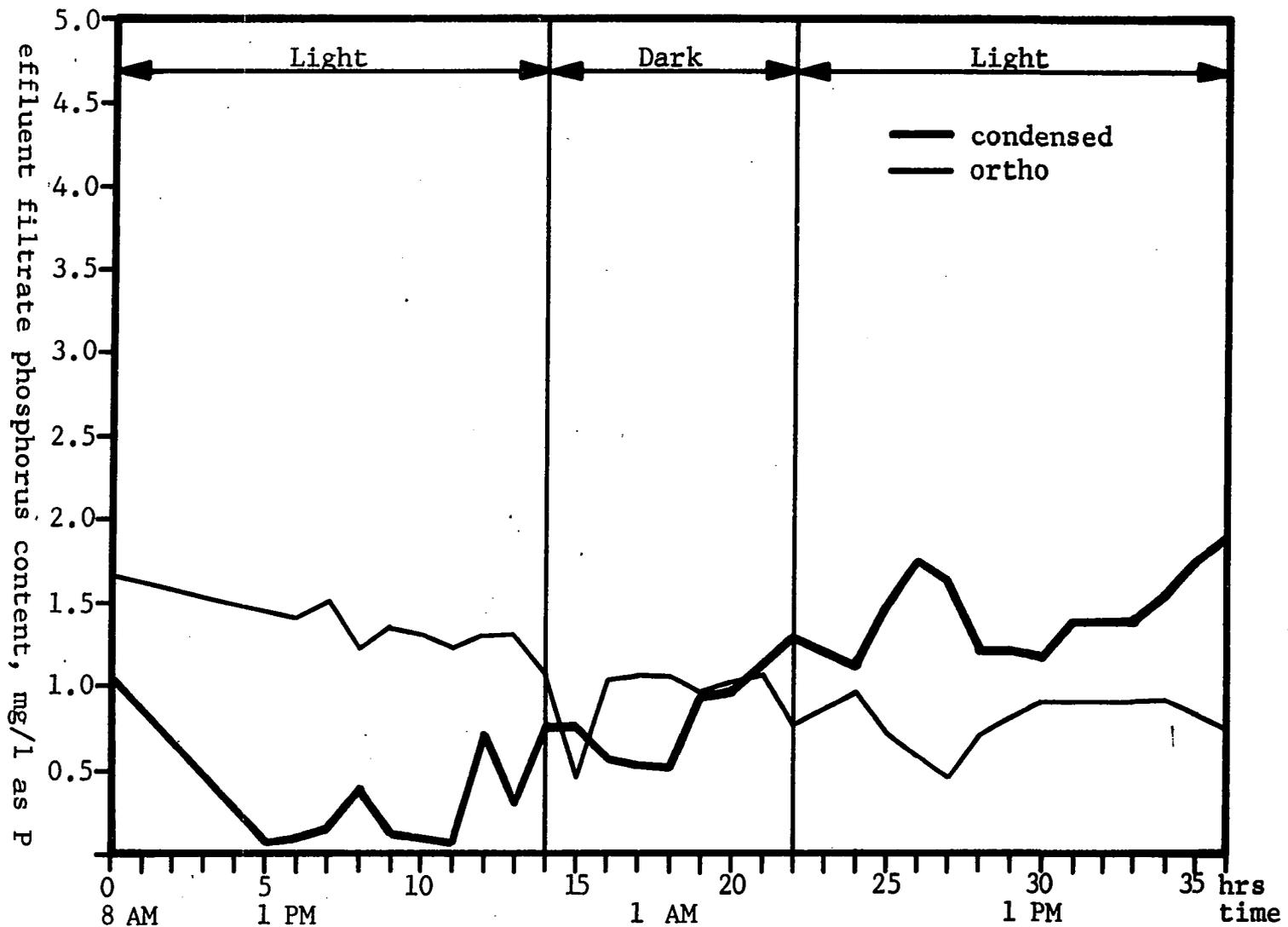
Figure 22. Phosphorus content of Chemostat effluent with Scenedesmus quadricauda. STPP added.
