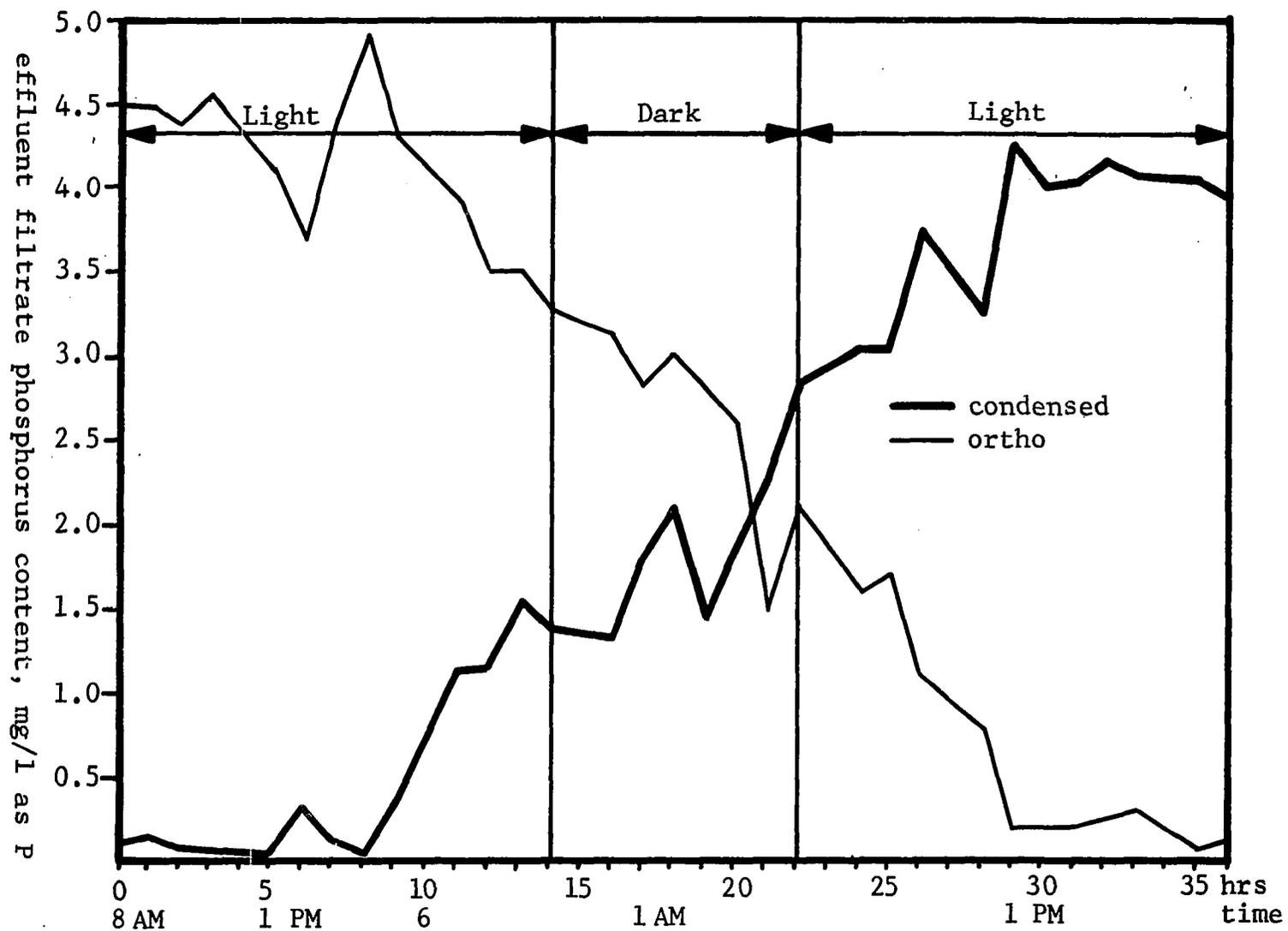
Figure 19. Phosphorus content of Chemostat effluent. Control run with SHMP added.
