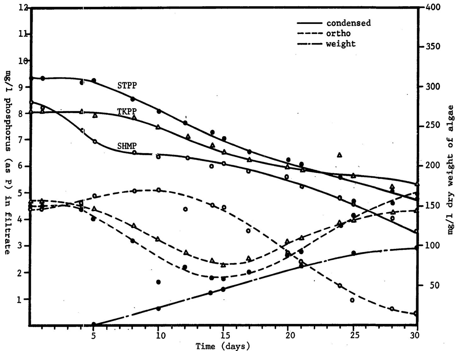
Figure 16. Effect of *Scenedesmus obliquus* on sodium tripolyphosphate, tetrapotassium pyrophosphate, and sodium hexametaphosphate in MSS medium with a typical growth curve for the organism.
