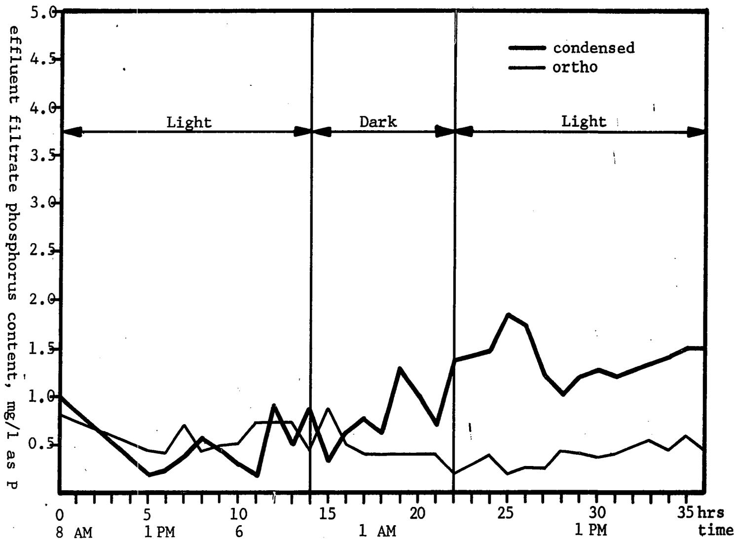
Figure 20. Phosphorus content of Chemostat effluent with Chlorella vulgaris. SHMP added.
