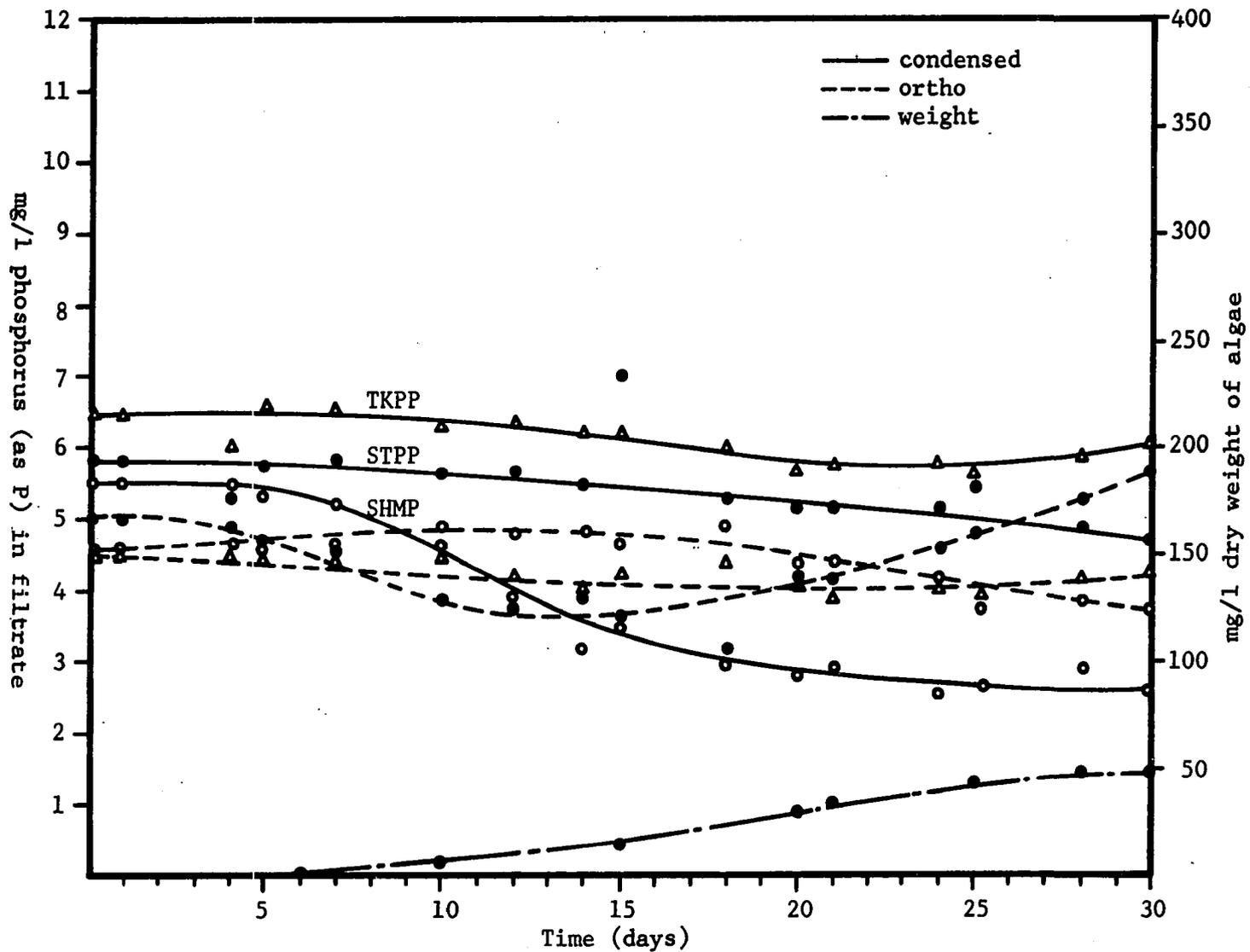
Figure 17. Effect of *Scenedesmus quadricauda* on sodium tripolyphosphate, tetrapotassium pyrophosphate, and sodium hexametaphosphate in MSS medium with a typical growth curve for the organism.
