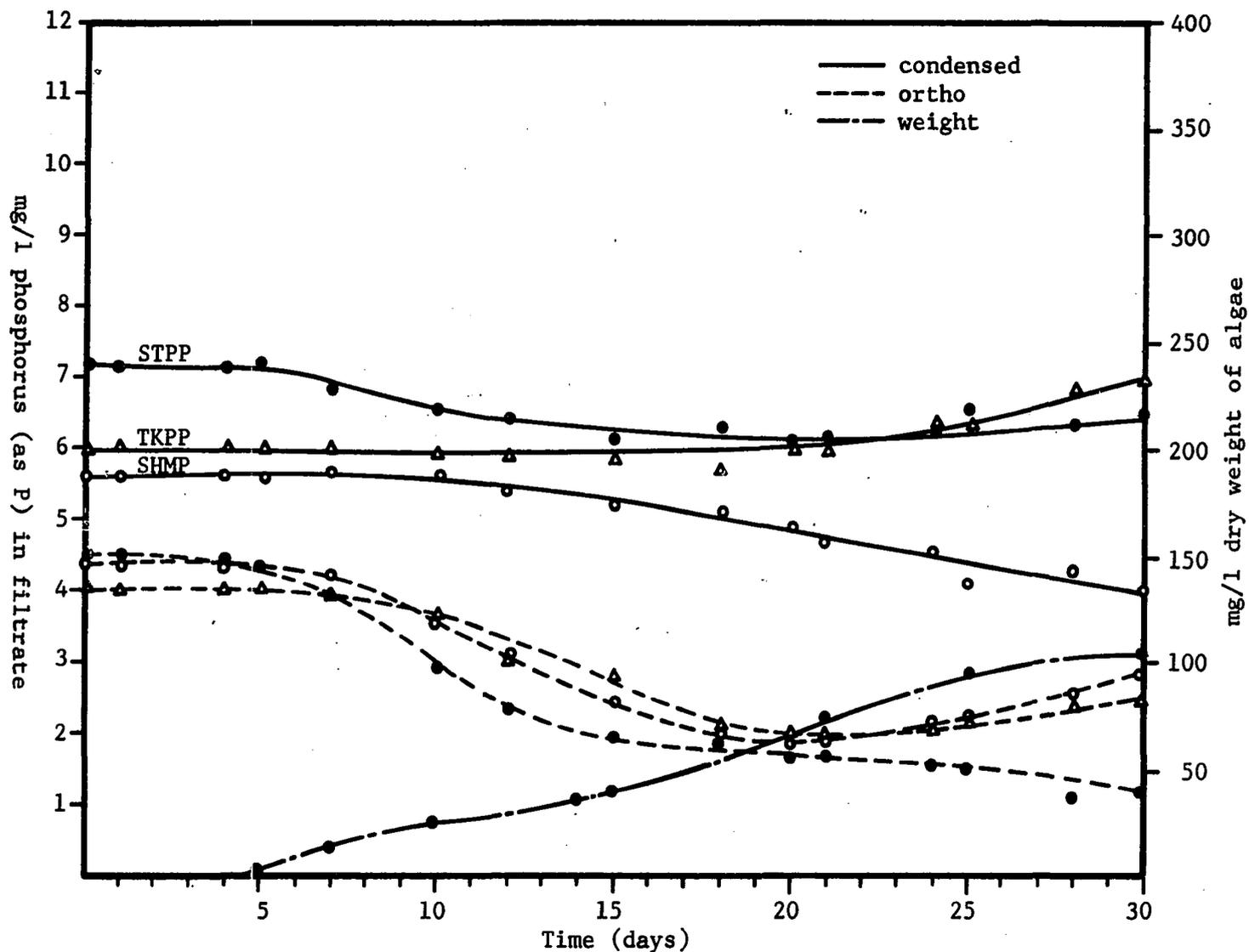
Figure 15. Effect of *Chlorella vulgaris* on sodium tripolyphosphate, tetra-potassium pyrophosphate, and sodium hexametaphosphate in MSS medium with a typical growth curve for the organism.
