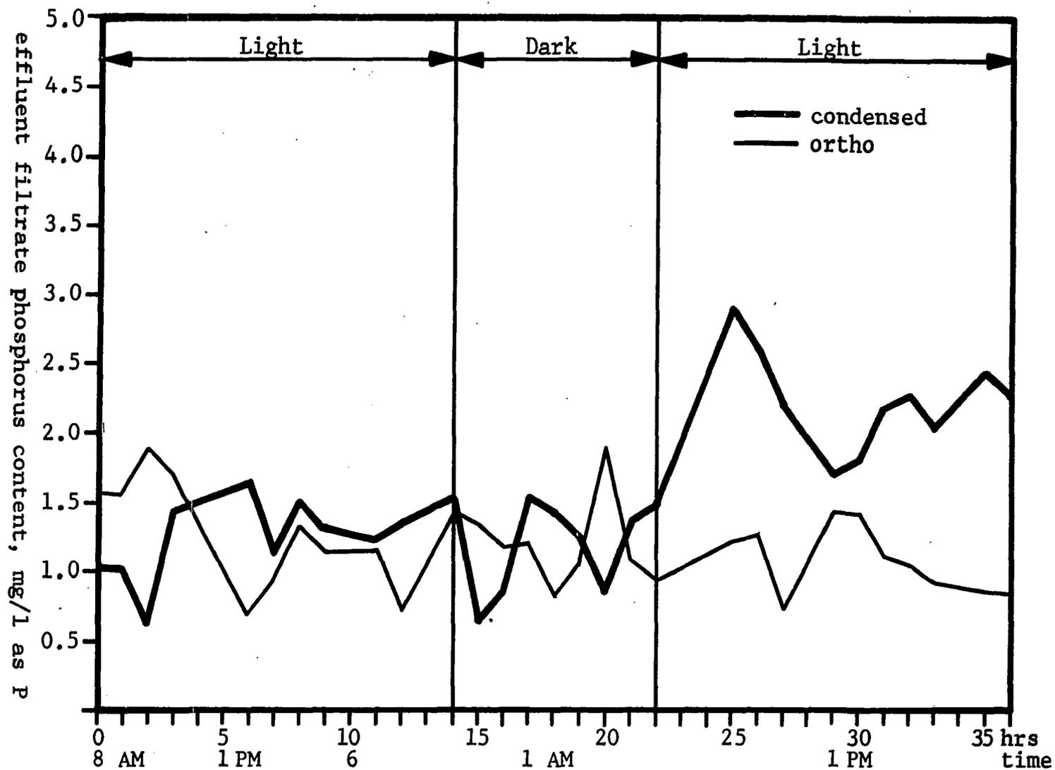
Figure 23. Phosphorus content of Chemostat effluent with Scenedesmus quadricauda. STPP added. Repeated run.
