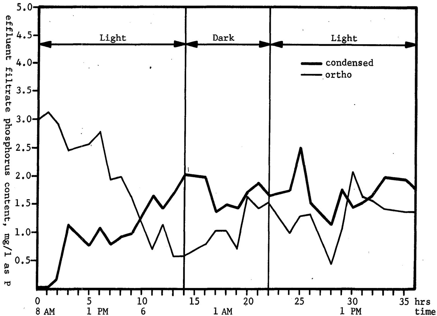
Figure 21. Phosphorus content of Chemostat effluent with Scenedesmus obliquus. SHMP added.
