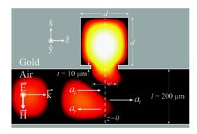
FIG. 1. (Color online) Schematic of a terahertz microcavity resonator side coupled to a metal waveguide overlayed with the simulated terahertz electric field from 2D-FDTD. The square resonator has side *d* and the coupling aperture has width *w* and thickness *t*. The terahertz electric field is polarized in  $\hat{y}$  direction and the waveguide is 200  $\mu$ m wide.
