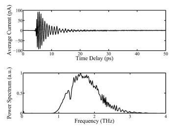
FIG. 3. Measured terahertz time-domain electric field waveform and accompanying power spectrum after propagation through a resonator structure  $(d=125 \ \mu\text{m} \text{ and } w=100 \ \mu\text{m})$ . The resonance dip at 1.331 THz is evidence of excitation of the resonator mode.
