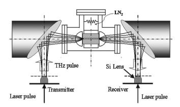
FIG. 1. Experimental setup for waveguide terahertz-TDS.
