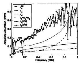
FIG. 4. Measured total amplitude absorption coefficient  $\alpha_t$  (c/a, dots) and  $\alpha_t$  (c/b, open circles) compared to the theoretical absorption  $\alpha_t$ . The theoretical absorption coefficient of the coaxial line  $\alpha_c$  and the measured Teflon  $\alpha_d$  are also shown. For comparison the theoretical absorption  $\alpha_c^{PP}$  is shown for the air-spaced, Cu PPWG. (Ref. 5).
