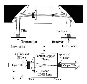
FIG. 1. THz-TDs arrangement and 2D quasioptical test structure.
