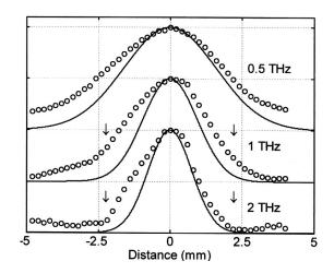
FIG. 3. Measured spatial cross section of the focus at the output edge of the THz electric field (normalized amplitudes) at various frequencies (open circles) and the calculated field dependence (solid lines).
