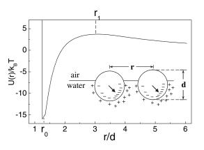
FIG. 1. Calculated interaction potential  $U(r)/k_BT$  as a function of r/d. Inset shows schematic distributions of surface charge and counterions near the water-air interface. The lateral asymmetry of the counterion clouds gives rise to a horizontal dipole moment in the plane of the interface.
