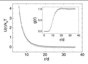
FIG. 3. Repulsive potential  $U(r)/k_BT$  vs r/d extracted from the measured g(r) shown in the inset. Approximately 10 000 images, each containing ~60 particles, taken at ~1 s intervals are used to calculate g(r) with ~100 nm spatial resolution. The area fraction occupied by the particles is  $n \approx 0.12\%$ . The solid curve shows the fitted function  $U(r)/k_BT = 879(d/r)^3$ .
