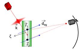
FIG. 1 (color online). Diagrammatic representation of a setup to detect the cooperative emission from a system of two identical two-level atoms. The atoms are driven resonantly by a weak laser of frequency  $\omega$  and propagation vector  $\vec{k}$ .  $\zeta$  is the angle between the laser propagation direction and the orientation of the atoms.  $\vec{d}_{eg}$  is the dipole moment of the atoms and  $\vec{r}_1$ ,  $\vec{r}_2$  are the position vectors of the atoms 1 and 2.
