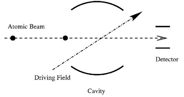
FIG. 1. The schematic arrangements for realizing quantum random walks. A continuous strong driving field inside the cavity can be applied by an external source. The time interval between two atoms in the atomic beam is selected larger than the interaction time in the cavity so that only one atom is presented inside the cavity at a time. The atoms are detected at the exit of the cavity by a state-selective detector.
