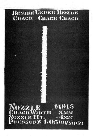
Figure 20. Broken Spray Pattern of Nozzle 14915 at a Height of 150 mm and a Crack Width of 5 mm
