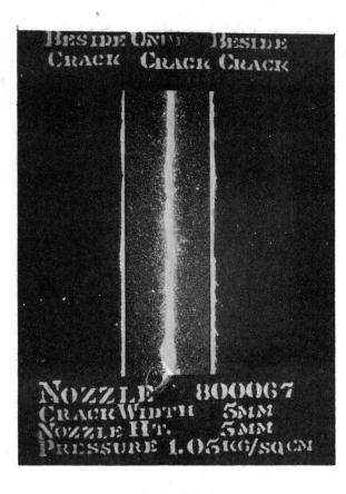
Figure 13. Spray Pattern of Nozzle 800067 at a Height of 5 mm and a Crack Width of 5 mm Using a Tank Pressure of 2.1 kg/cm<sup>2</sup>
