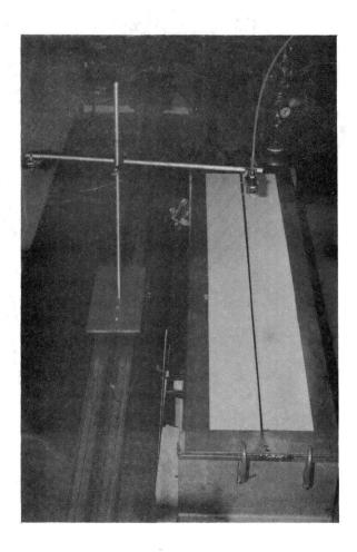
(2 mm and 5 mm), (2) three nozzle types (Spraying Systems Multi-Teejet<sup>®</sup> nozzle 800067, Spraying Systems Crack and Crevice nozzle 14915, and a B & G 100 C.C. Crack and Crevice tip extension), (3) four nozzle heights (4 mm inside the crack and 5 mm, 75 mm, and 150 mm above the crack) and (4) two tank pressures (1.05 kg/cm<sup>2</sup> and 2.1 kg/cm<sup>2</sup>). The test was conducted at various application speeds.
