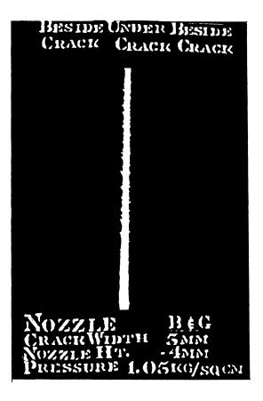
Figure 15. Spray Pattern of the B & G Nozzle at a Height of - 4 mm Inside the Crack and a Crack Width of 5 mm Using a Tank Pressure of 2.1 kg/cm<sup>2</sup>
